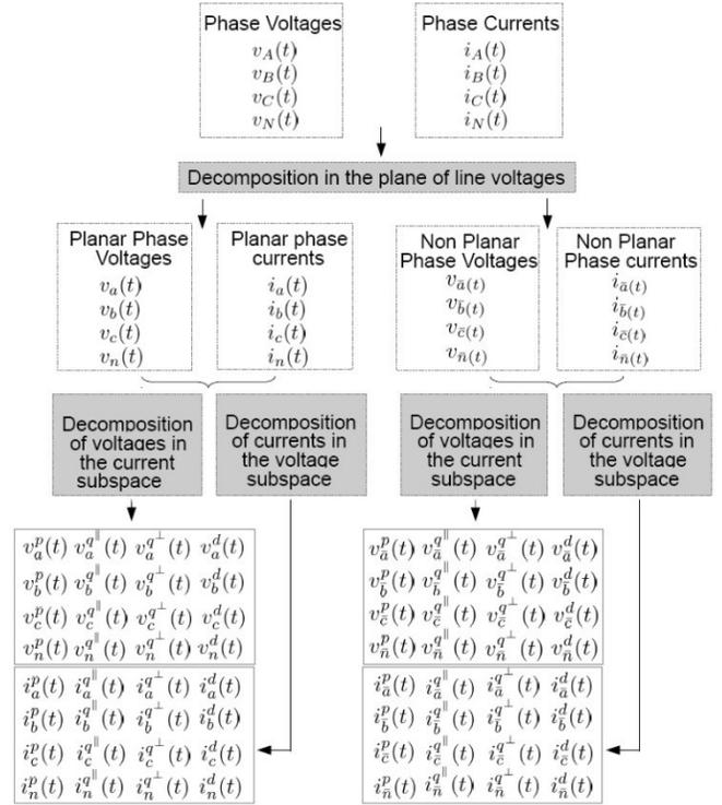
Fig. 3. Schematic diagram of the decomposition process by orthogonal components.
