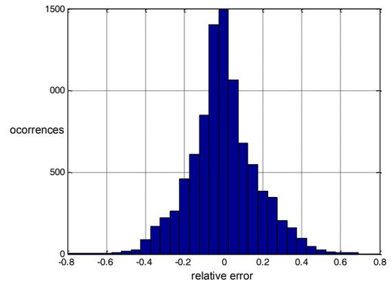
Fig. 4. Histogram of the relative error in relation to the fault distance estimation by the fuzzy system using test data.
