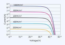
Average efficiency reduction of 4.5% at  $200 \text{W/m}^2$  according to EN 60904-1.
