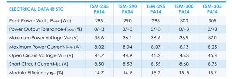
Values at Standard Test Conditions STC (Air Mass AM1.5, Irradiance 1000W/ $m^2$ , Cell Temperature 25°C). Power measurement tolerance:  $\pm 3\%$
