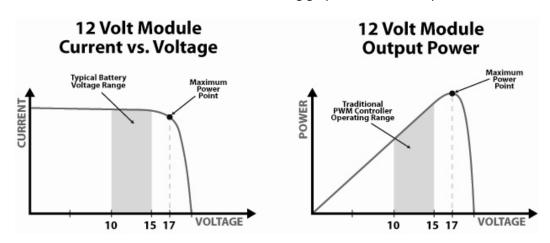
Because these traditional controllers rarely operate at the  $V_{mp}$  of the solar array, energy is wasted that could otherwise be used to charge the battery and power system loads. The greater the difference between battery voltage and the  $V_{mp}$  of the array, the more energy is wasted.
