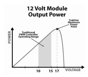
A consequence of this is: the less charged the batteries are (lower battery voltage), the more "boost" current they will receive. This is precisely the time when batteries will benefit from an increased amount of charging current.
