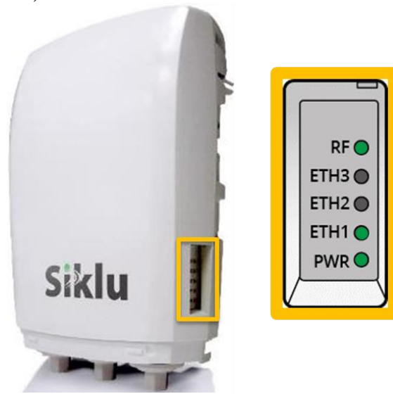
Figure 5: MultiHaul™ T200 - front view and LEDs
