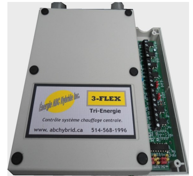
Fig.1 3-FLEX add-on controller enhances house thermostat aux. heat control capabilities.
