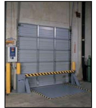
The Serco Dock Guard™ Safety Gate is powered by a simple linear actuator. An adjustable counter-balance spring provides controlled descent of the barrier arm. Proximity switches safely monitor its position.
