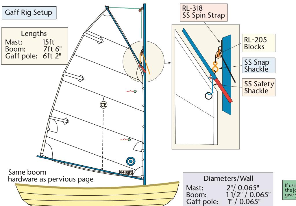
If using .058" wall tubing, overlap the joint 12". Two 8 footers will give you 15ft.
