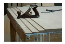
Cut the slope of the scarph evenly over the whole stepped surface. As you go, the scarph will start to appear as a series of lines as the plane cuts through the different veneers in the plywood. These lines are similar to contour lines on a map, and you will find that they give an excellent visual guide to how evenly you are cutting. Below is a photo of the scaphs as they appear close to the end of the cutting process.
