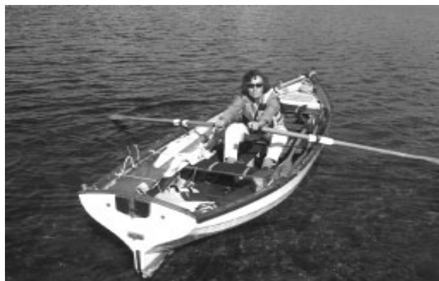
Marcia Mullins rowing using Douglas oarlocks with Barkley Sound round-loomed oars and Dreher sleeves and buttons.
