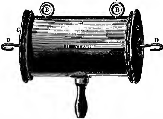
FIG. 178.—Stethograph. A, Metal drum; B, hooks for tapes which pass round neck; C, rubber discs; D, hooks for attaching tapes which are tied round thorax; E, tube leading to the recording tambour.
