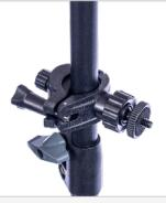
4. Close the clamp around the top extension pole, near the connection with the vertical locking knob. Swing the side knob back into the locking arm and tighten to hold the clamp in place. Adjust the mid-mount knob on this clamp if needed to secure the position on the pole.
