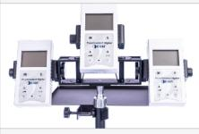
12. Mount the EAI Pointoselect devices into the device clamps by loosening the device clamp knob, inserting the device, and tightening the knob until the device is secure in the clamp. Repeat for each device until all devices are locked in place.
