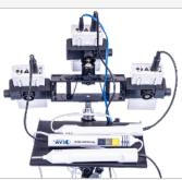
13. Plug into each EAI Pointoselect device the handset that will be used. Be sure to include the grounding bar with each Point Probe handset. The handsets can be positioned on the stand shelf, and the wires can be placed over the hook to allow them to hang cleanly from the stand.
