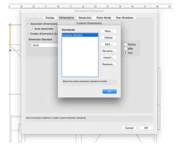
After naming the standard, the Edit Custom Dimension Standard dialog will appear. At the top of this dialog, offsets and lengths of the various parts of a dimension can be set.
