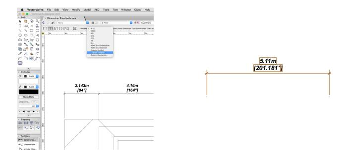
One final note. When placing dimensions using a dual dimension standard, you can override the default dual view setting from the standard. With the dimension selected, in the Object Info palette you can toggle between Primary Only, Secondary Only, or Both. This allows you to choose which dimension text to show, per dimension object.
