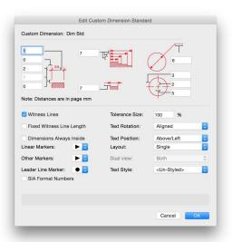
By default, all dimensions will have a dimension standard. With a dimension selected, if you look in the Object Info palette under the Shape pane, you see the Dim Std field. This dimension is using the arch standard. If we change it to ISO, you will see the appearance of the dimension change to reflect the ISO standard settings.
