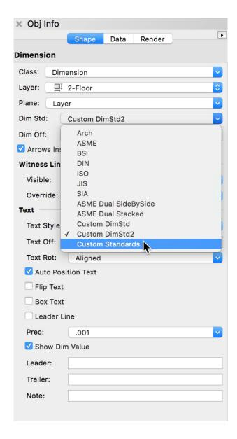
If we set it to Dual - Stacked, this standard will show two dimensions using different unit settings. This configuration will show the dimension text, one stacked above the other. Under Dual View, you can choose the default visibility for the dual dimensions. You can choose to show only the primary dimension, only the secondary dimension, or both.
