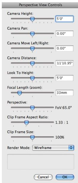
Now the camera is at the desired height, but it is tilting down slightly. To correct this, go to the **Look To Height** slider, and in the white data box enter the same height we entered previously:
