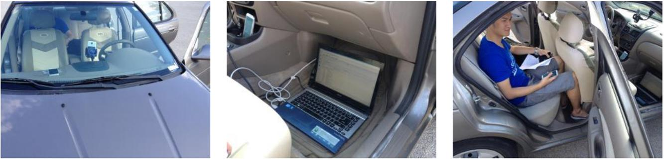
**Figure 2: Eight Samsung (Android) smartphones placed at various positions in the car during the data collection phase. One phone taped to the dashboard to gather data not polluted by the wobbling of the phone. Also, middle figure shows the OBD connected to the car and laptop.**
