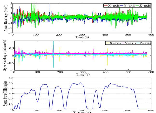
**Figure 1: (a) Accelerometer and (b) gyroscope data when phone placed in the cup holder and driving in the university town. (c) OBD data captured from the same car trips.**
