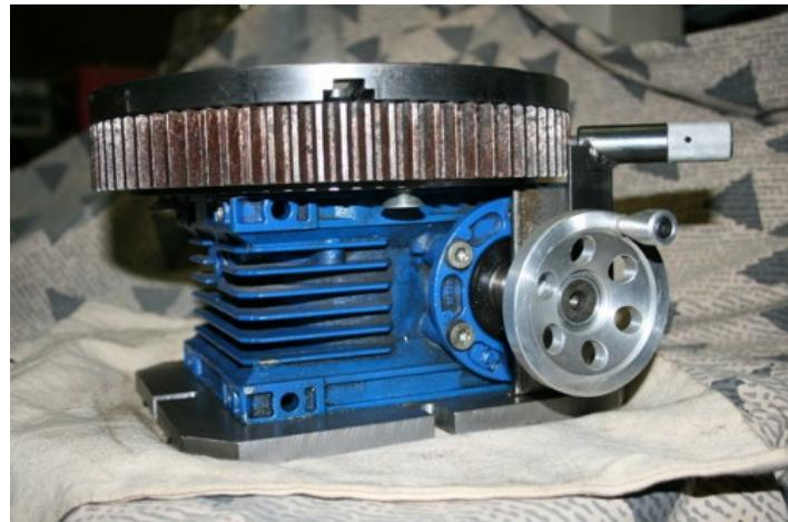
Homemade rotary table utilizing a right-angle wormbox with an 80:1 reduction. Features a 10" diameter top plate.
