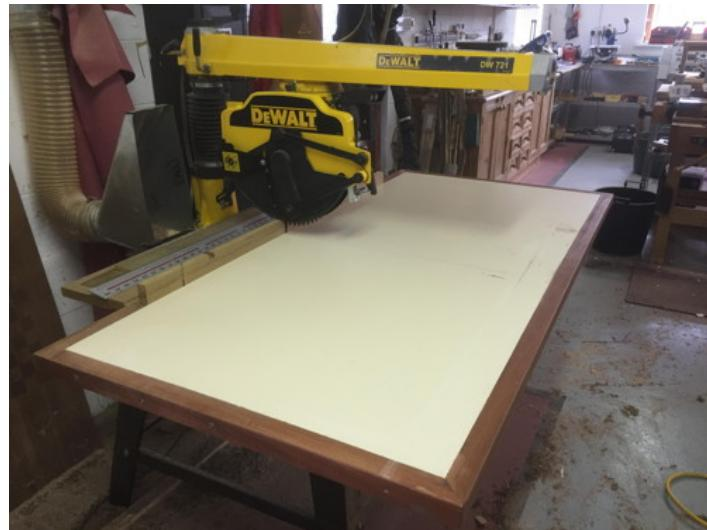
Homemade radial arm saw table constructed from melamine-faced particle board.
