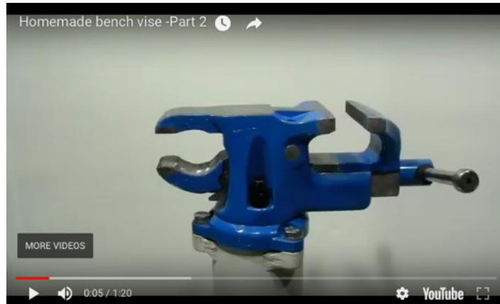
Homemade bench vise constructed from steel stock.
