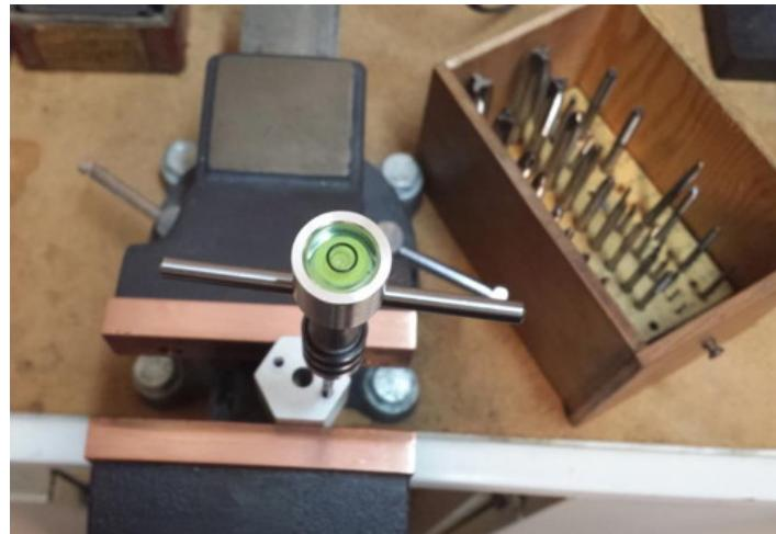
Homemade tap handle bubble level constructed from 6016 aluminum stock and off-the-shelf bubble levels.
