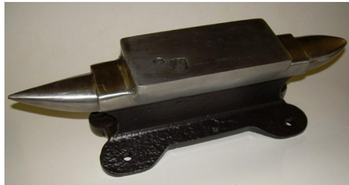
Homemade anvil constructed from a surplus railroad section.
