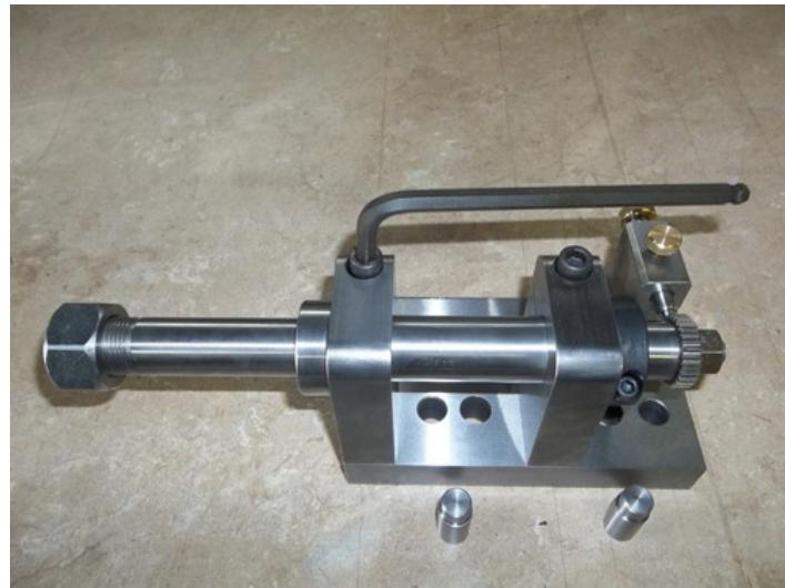
Homemade indexing fixture intended to facilitate the process of fabricating #3 module gears.
