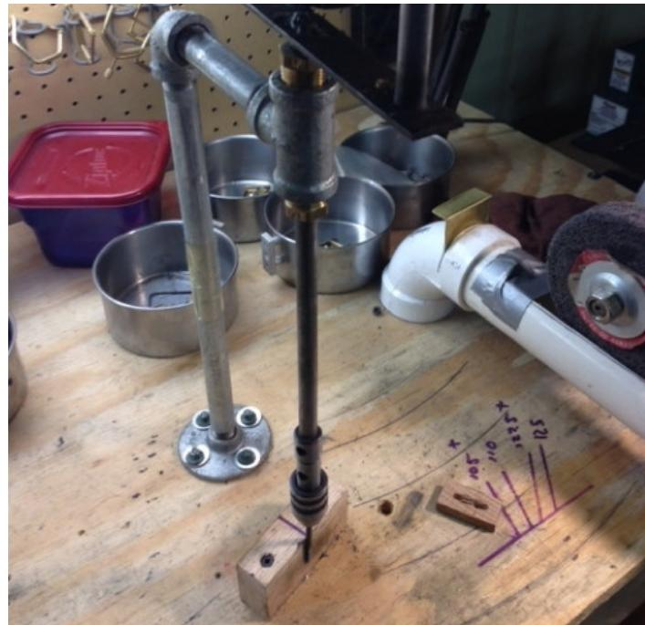
Homemade tapping machine constructed from GI pipe and fittings, a tap holder, and brass bushings.
