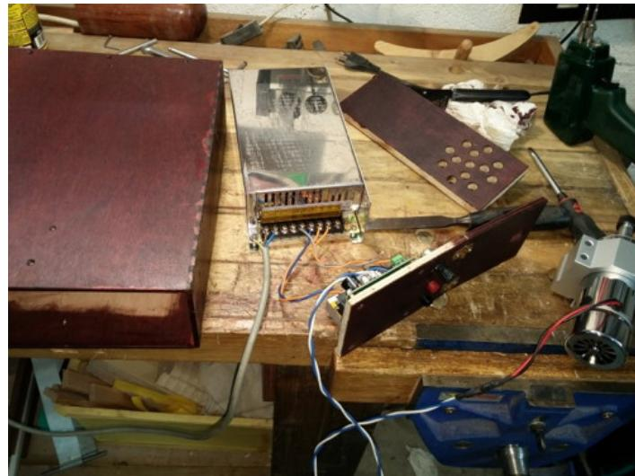
Homemade high speed spindle constructed from an off-the-shelf spindle kit, ER11 chuck, and a homemade wooden box.
