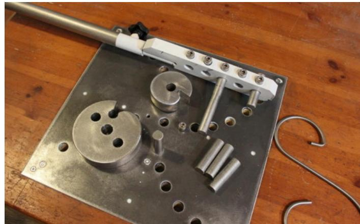
Homemade bar bender constructed from bar stock, steel plate, and steel dowels.
