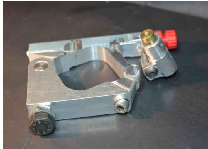
Homemade laser aligner constructed from a surplus laser, steel stock, batteries, nuts, and bolts.
