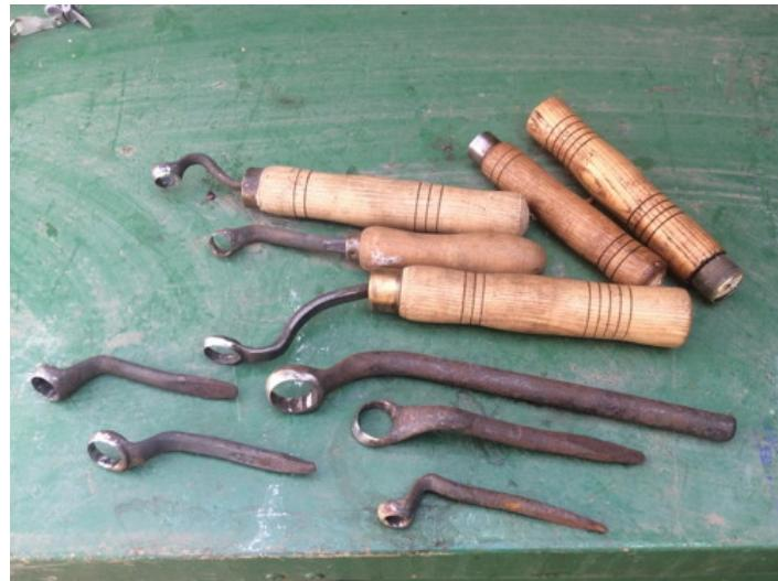
Homemade scorps constructed from surplus box wrenches and lumber.
