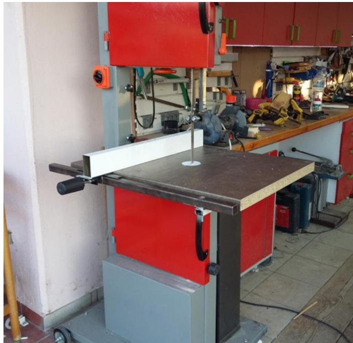
Homemade bandsaw constructed from tubing, bearings, sheetmetal, and an electric motor.
