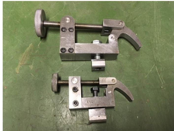
Homemade claw clamps constructed from steel stock, threaded rod, and screws.
