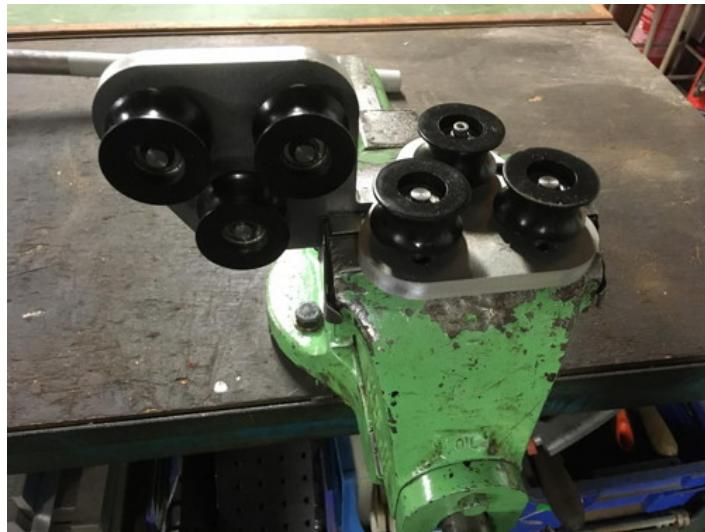
Homemade coiled tube straightening tool constructed from steel plate and off-the-shelf bobbins.
