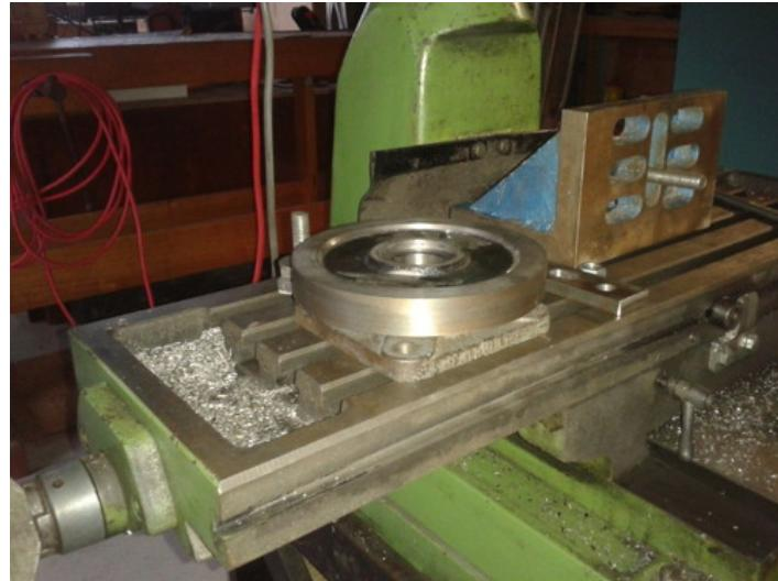
Homemade manual rotary table constructed from a flange bearing and a gym weight.
