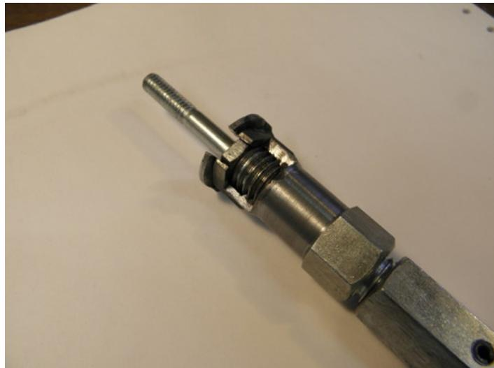
Homemade finger saver screw holder constructed from a coupling nut, set screw, threaded rod, and a washer. Used to hold bolts being deburred or sanded.
