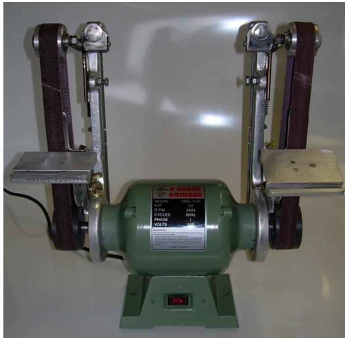
Homemade twin belt sander constructed from an electric motor, homemade aluminum castings, bar stock, springs, and contact wheels.
