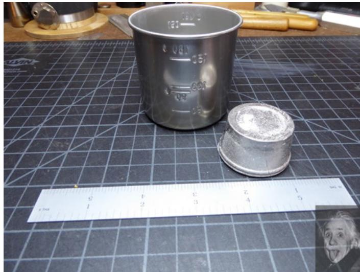
Homemade plug gauge constructed from Cerrosafe. Used by gunsmiths to measure internal diameters, it can also be used as a dimensional cast for measuring any hole diameter.
