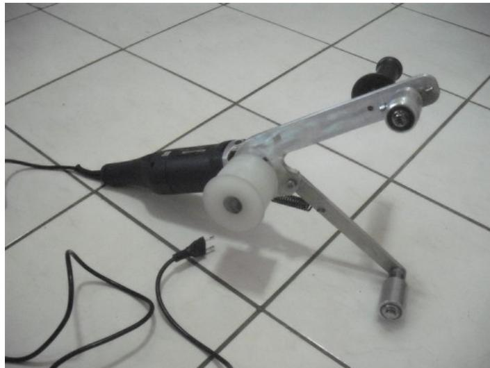
Homemade portable belt grinder powered by a rotary tool.
