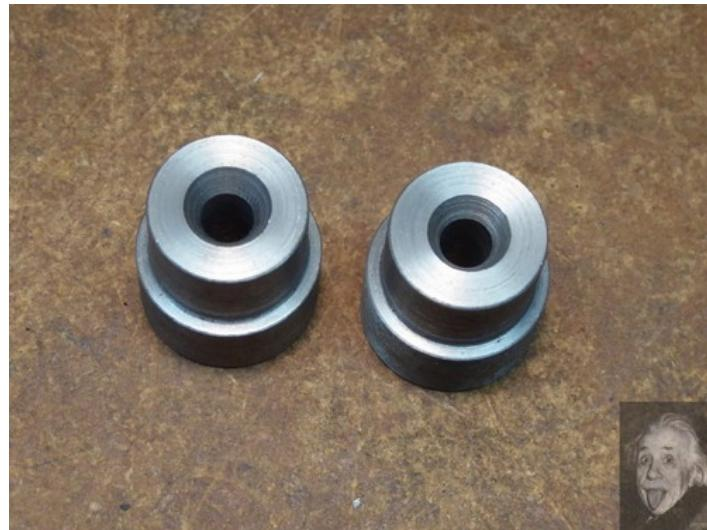
Homemade tailstock alignment buttons constructed from round bar stock.
