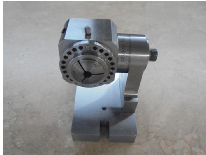
Homemade tilting dividing fixture constructed from 4140 steel and cap screws.
