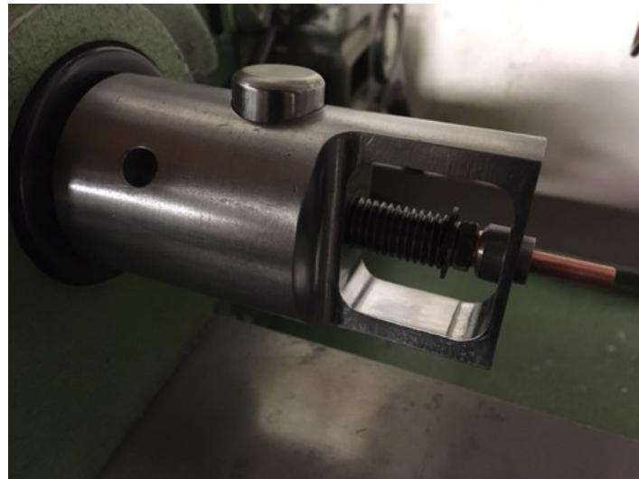
Homemade lantern chuck constructed from steel and bar stock. Constructed to facilitate the threading of copper rivets.
