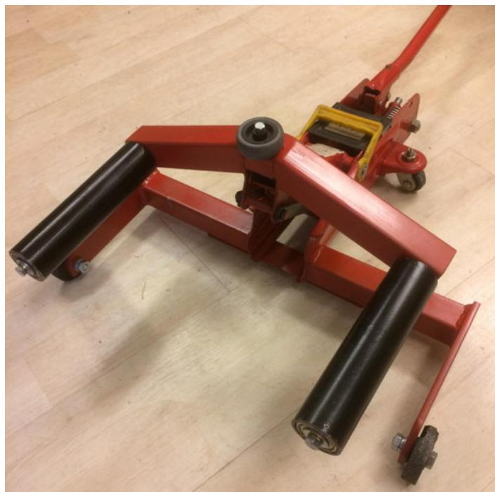
Homemade tire lift constructed from a surplus floor jack, tubing, bar stock, and bearings.
