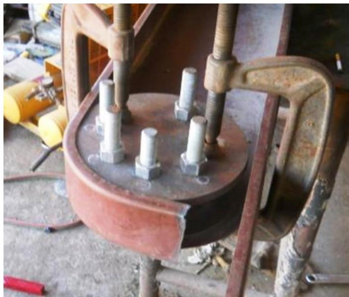
Homemade adjustable round forming anvil constructed from steel plate, threaded rod, and nuts.
