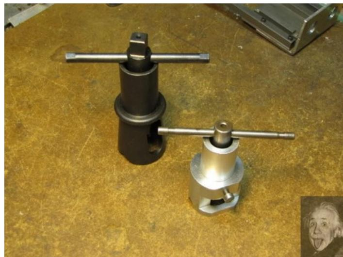
Homemade tap wrench guide constructed from aluminum and a screw.
