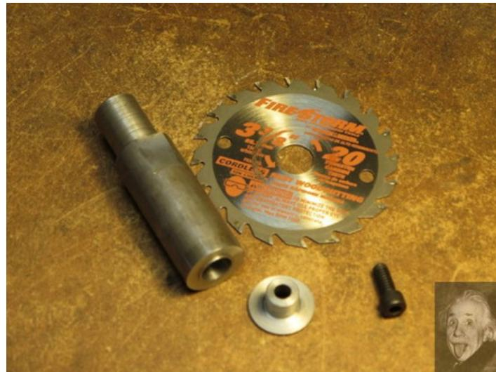
Homemade low-profile slitting saw arbor featuring a top hat only .080" thick enabling operation within .1" of the vise.
