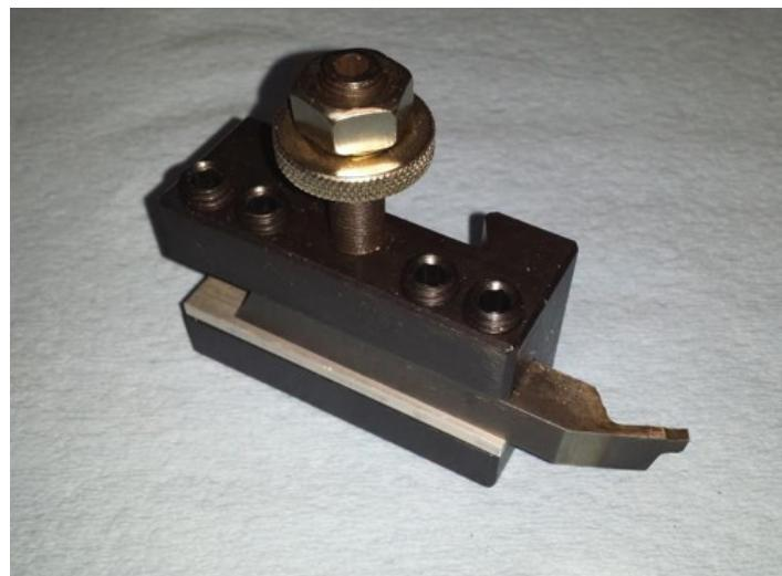
Homemade groove and trepanning tool
