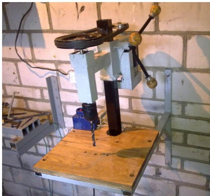
Homemade drill press constructed from tubing, shafting, bearings, a chuck, pinion gear, pulley, bar stock, and a surplus washing machine motor.
