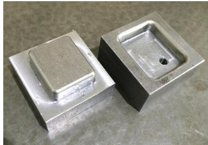
Homemade sheetmetal former constructed from steel stock. Used to form a lubricator body and lid for a scale model steam wagon.
