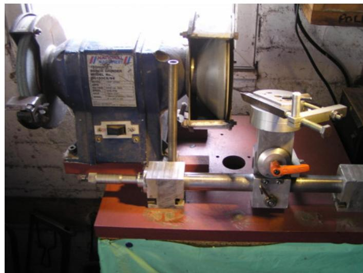
Homemade tool sharpener constructed from a surplus bench grinder, steel baseplate, bar stock, and a dial indicator.
