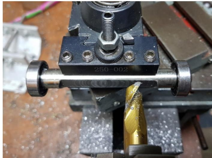
Homemade lathe truing tool constructed from shafting, bearings, and Allen bolts.
