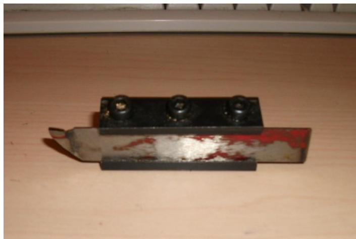
Homemade parting tool adapted from a surplus tungsten carbide-tipped (TCT) saw blade. Capable of being readily sharpened on a green grindstone.
