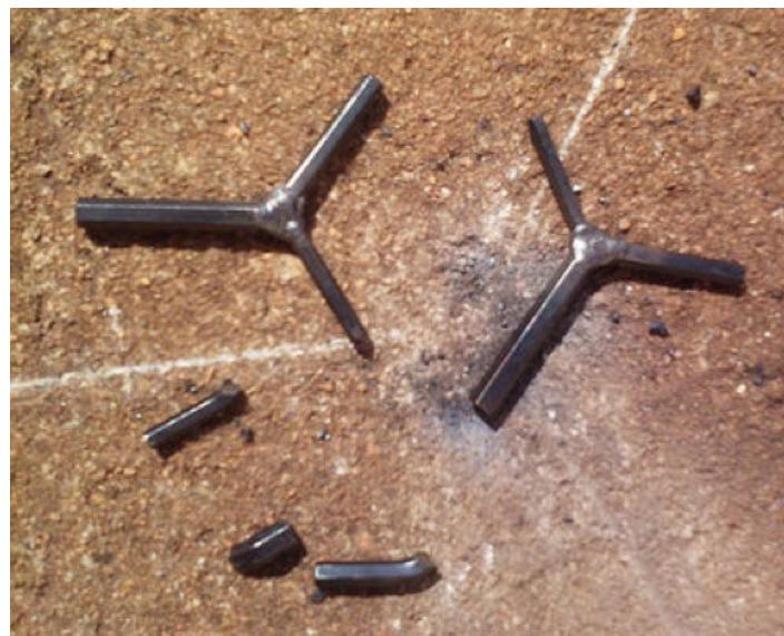
Homemade Y Allen wrenches constructed from surplus Allen wrenches.
