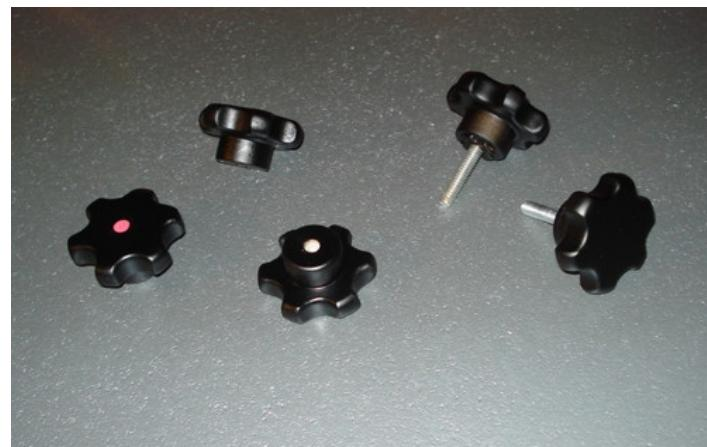
Homemade threaded knobs fashioned from MDF. Lathe and router table were utilized for rounding. Finished with sealant and black enamel.
