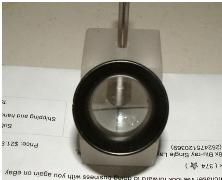
Homemade optical punch constructed from a polycarbonate block, surplus magnifier, and a drill blank.
