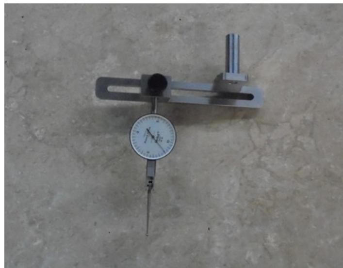
Homemade dial indicator attachment constructed from O1 and 12L14 steel stock.
