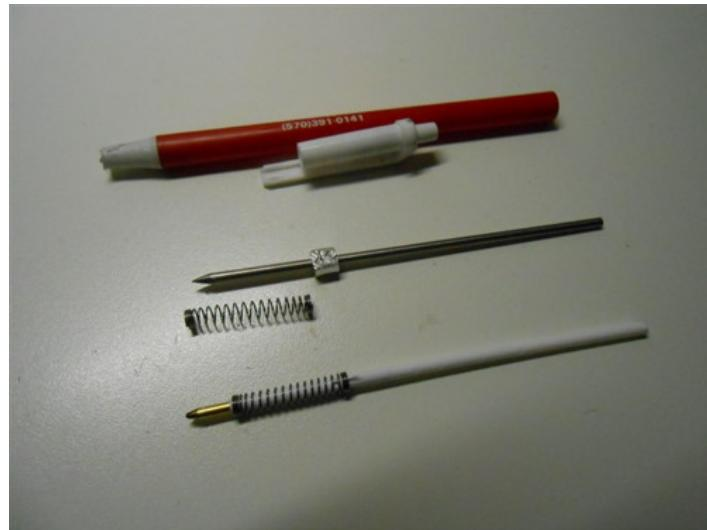
Homemade retractable scribe constructed from a retractable pen and a metal scribe.
