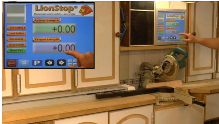
Homemade automatic miter saw stop constructed from a rail, bearings, servo, driver, a surplus laptop and touch monitor. Off-the-shelf components include a 5-axis CNC board and a stepper driver.
