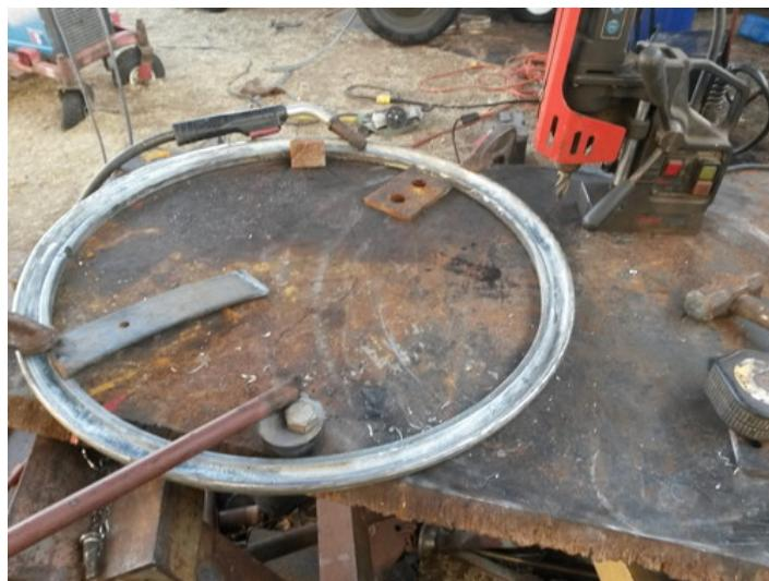
Homemade truck wheel ring straightener constructed from a length of bar stock and a cam bolted to the work table.
