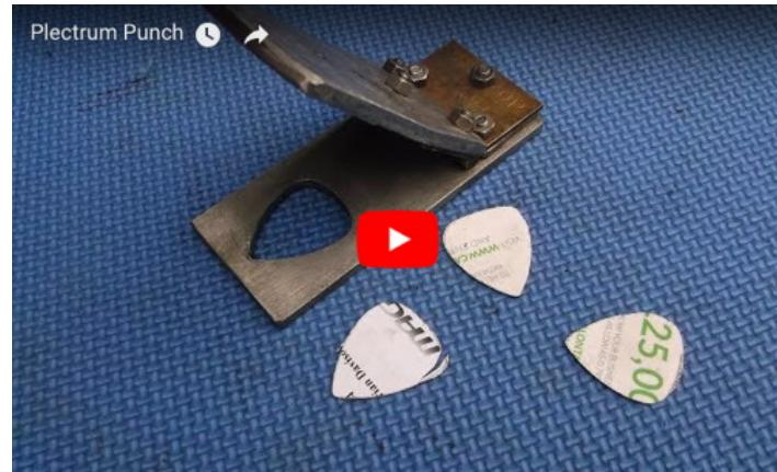
Homemade plectrum punch constructed from mild and tool steels, and a brass hinge.
