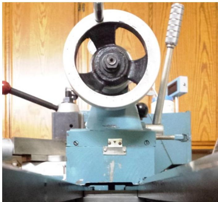
Homemade tailstock clamp improvement for a 12" x 37" lathe. Intended to prevent the tailstock slipping from its clamped position when drilling large-diameter holes. Cast iron clamping plate was replaced with CRS.
