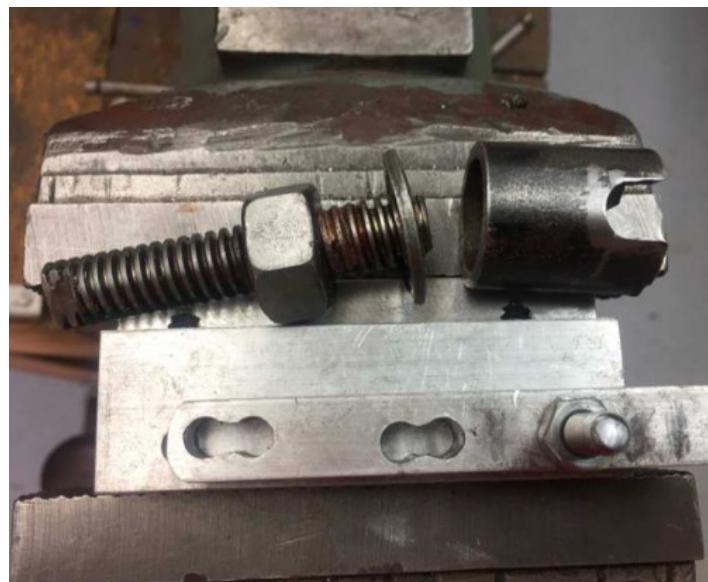
Homemade nut tightening tool constructed from tubing and threaded rod.
