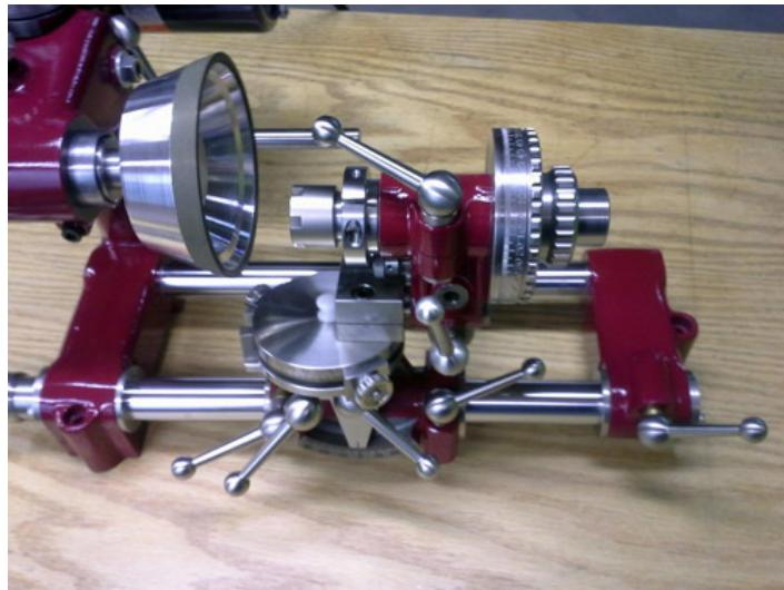
Homemade tool and cutter grinder
