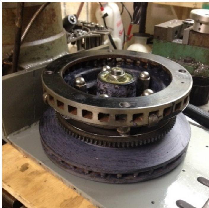
Homemade rotary table constructed from a pair of surplus brake rotors, steel plate, sheetmetal, a lawnmower ring gear, and homemade spindle and worm gear.
