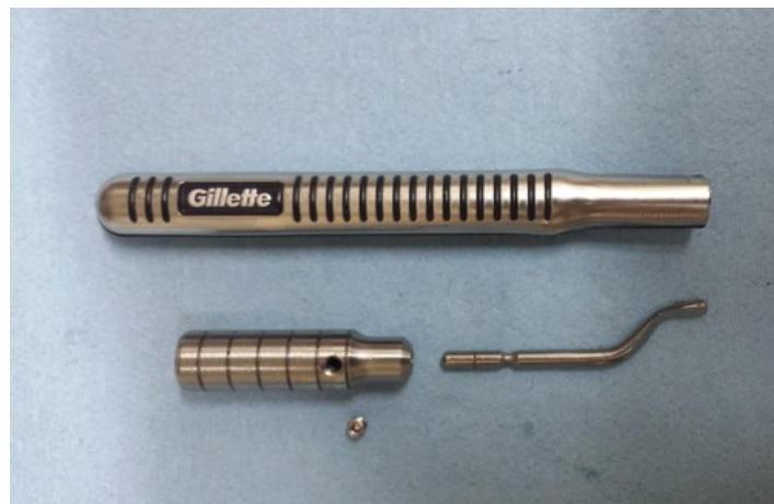
Homemade deburring tool adapted from a surplus razor handle. Head was turned from 303 stainless rod stock.
