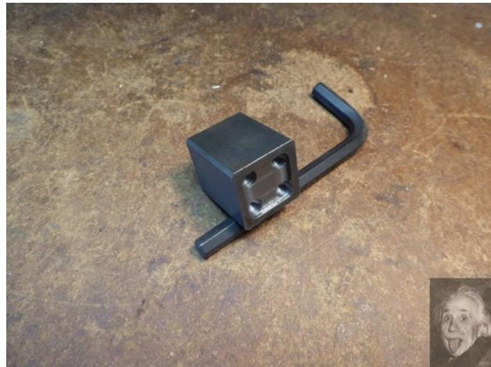
Homemade lathe height gauge constructed from a steel block.
