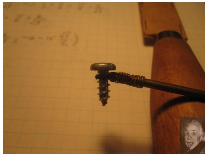
Homemade screw garrote fashioned from brass tubing, wire, and waxed thread. Intended to facilitate the process of securing a screw while it's being started.
