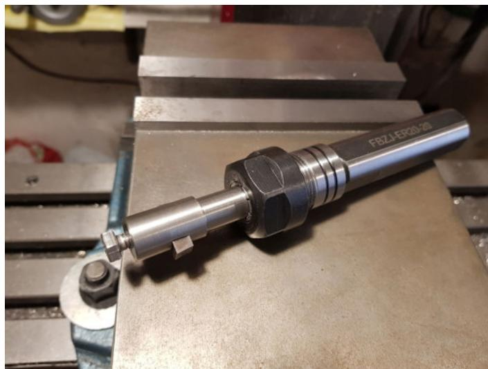
Homemade keyway cutter constructed from stainless steel bar stock. Can be used on a lathe or drill press.
