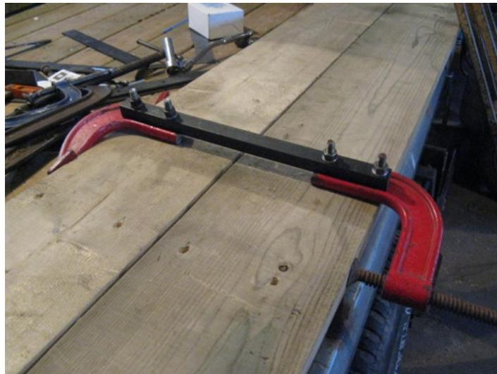
Homemade c-clamp modification consisting of utilizing a bolt-on extension to add 7" of throat depth to the clamp.
