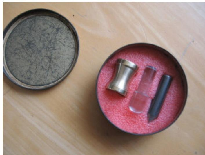
Homemade optical center punch fashioned from brass, acrylic, and medium carbon steel.
