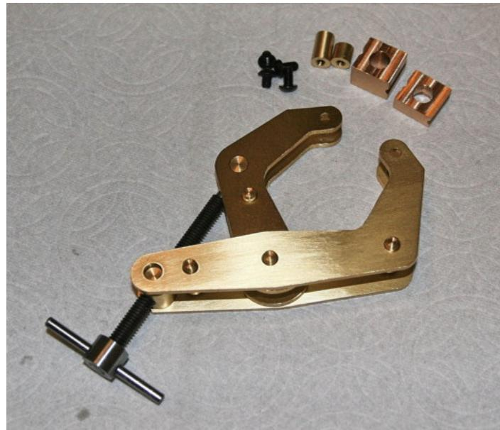
Homemade brass Kant twist clamp constructed from brass, copper, and steel rivets. Lead screw is constructed from Grade 8 threaded rod.
