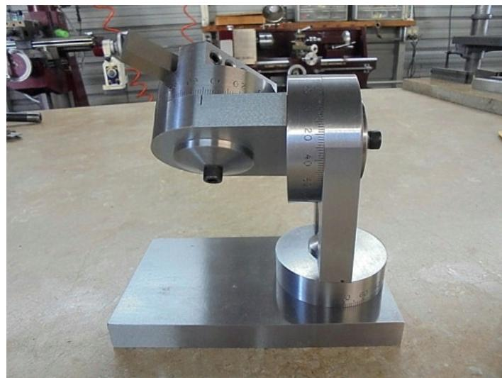
Homemade universal grinding fixture constructed from 4140 steel.
