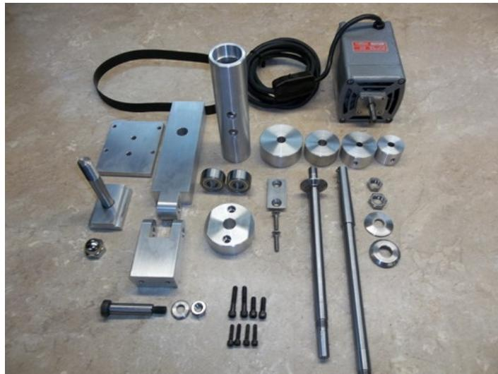
Homemade tool post grinder constructed from a surplus high speed motor, angular contact bearings, spindle, and homemade aluminum pulleys.
