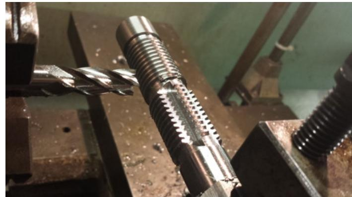
Homemade worm gear hob constructed from 304 stainless steel hex stock.
