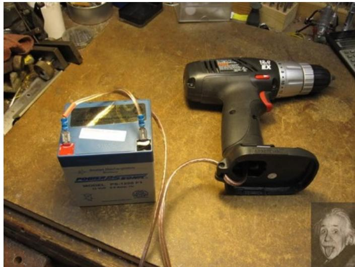
Homemade cordless drill extension constructed from a small lead-acid battery, wire, and connectors.
