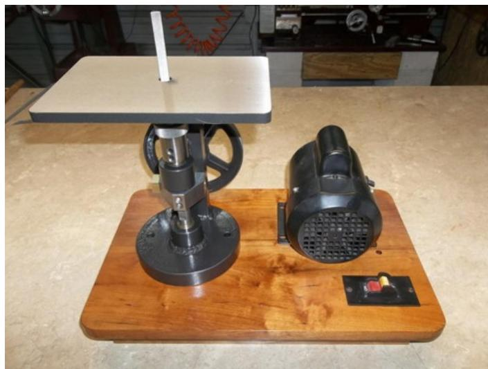
Homemade filing machine constructed from steel, ball bearings, set screws, and a cherry wood base. Intended to facilitate the process of maintaining squareness when filing 90-degrees from a flat surface.
