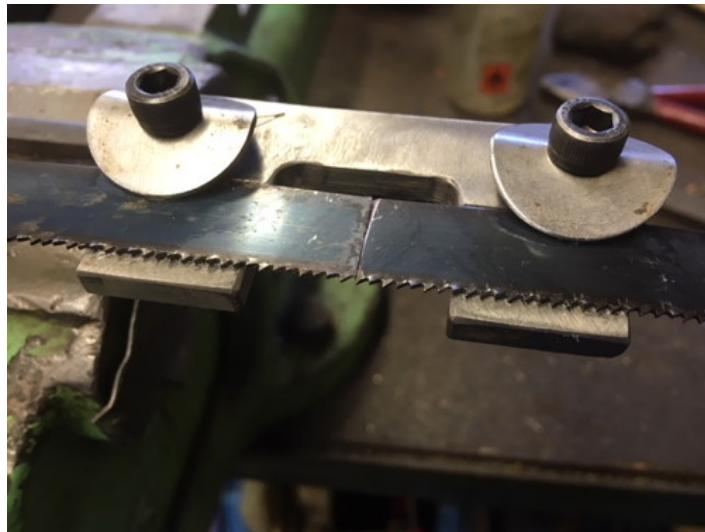
Homemade bandsaw blade soldering fixture constructed from steel stock, washers, and bolts. Mounts on a vise.
