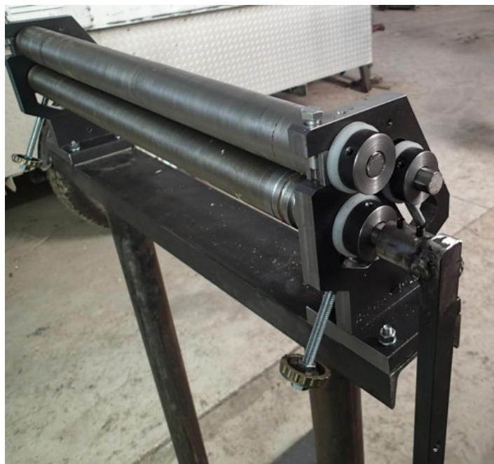
Homemade slip roller constructed from steel plate, tubing, gears, bearings, threaded rod, and knobs.
