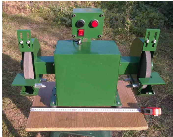
Homemade bench grinder constructed from a surplus electric motor, sheetmetal, and bar stock.
