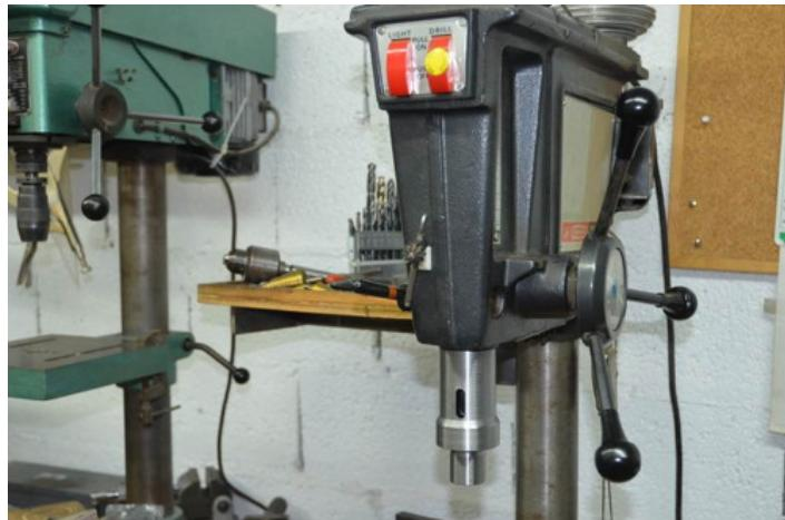
Homemade morse taper for drill press constructed from a surplus R8 to MT2 sleeve and bearings.
