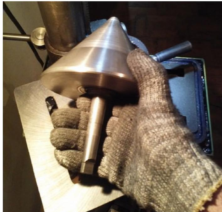
Homemade pipe center constructed from steel stock, an arbor and a bearing.
