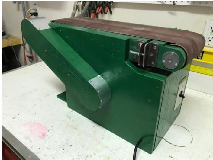
Homemade belt sander constructed from a bench grinder, plywood, angle iron, and steel plate.
