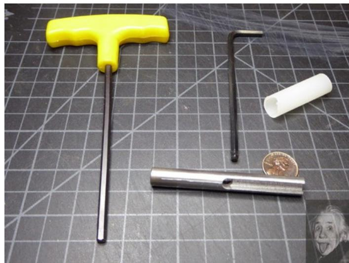
Homemade Allen wrench handle constructed from round bar stock and plastic tubing. Gives L-shaped wrenches better handling and torque.
