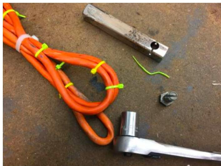
Homemade cable tie tightener constructed from square tubing and a bolt.
