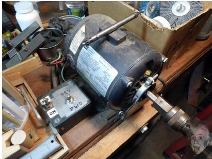
Homemade bench motor constructed from a reversible electric motor and a chuck.
