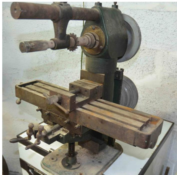
Homemade horizontal milling machine
