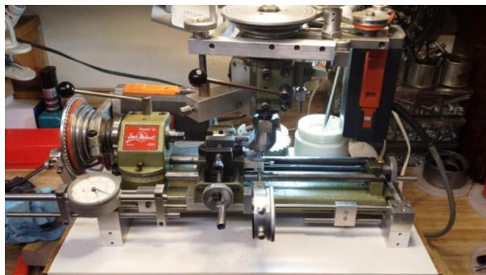
Homemade lathe modifications intended for a Unimat SL1000 including: a storage platform and drawer, tapped holes for future enhancements, dial indicators, adjustable carriage stops, and up-rated motors.
