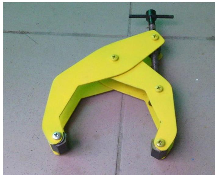
Homemade Kant twist clamp constructed from steel plate, bar stock, and threaded rod.
