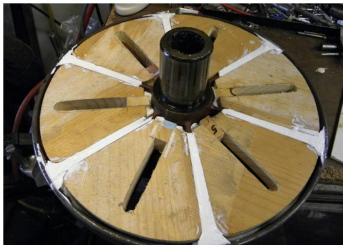
Homemade drill press table modification constructed from lumber and caulk.
