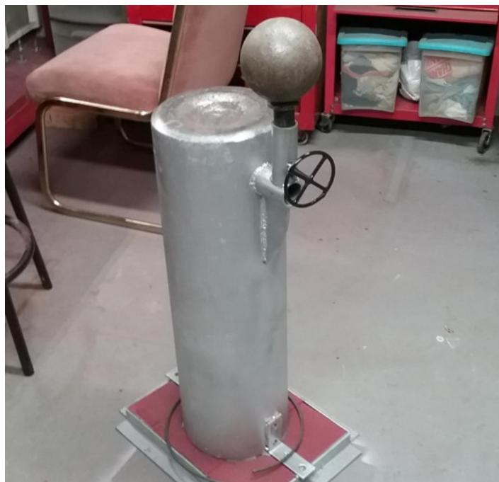
Homemade dishing stump constructed from a surplus gas bottle. Accessory arm allows forming tools to be attached.
