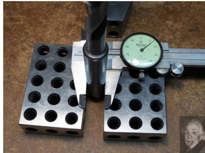
Homemade taper measuring method constructed using 123 blocks.
