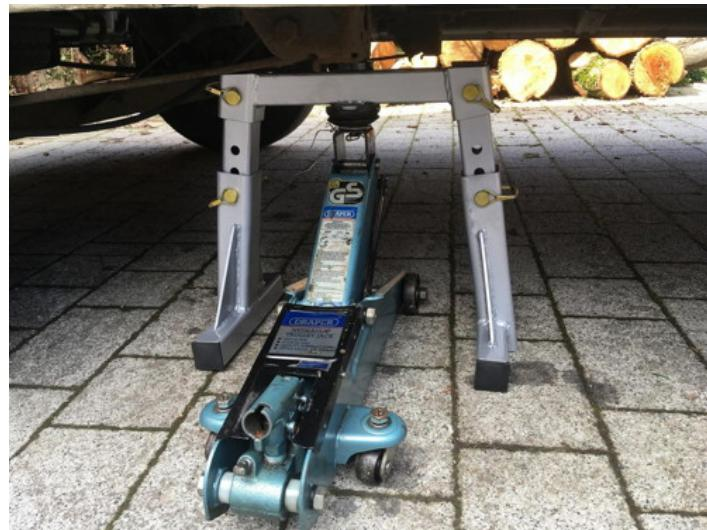
Homemade axle stands constructed from tubing and steel pins. Provides an extra measure of safety when lifting a vehicle.
