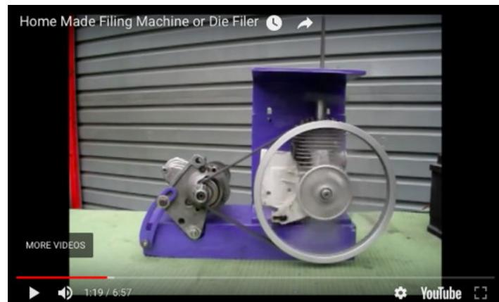
Homemade filing machine constructed from surplus chainsaw components, pulleys, and a surplus H-beam section.
