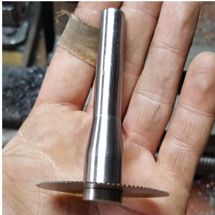
Homemade slitting saw arbor constructed from surplus round bar stock.
