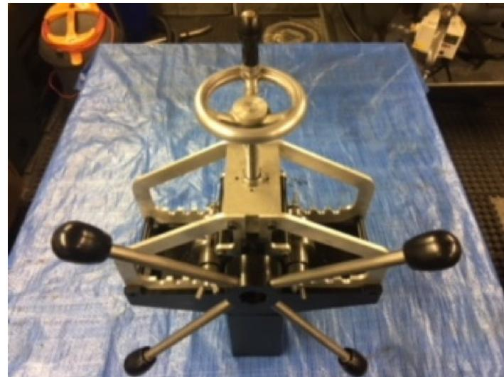
Homemade ring roller constructed from steel stock, aluminum, bearings, knobs, bolts, circlips, and threaded rod.
