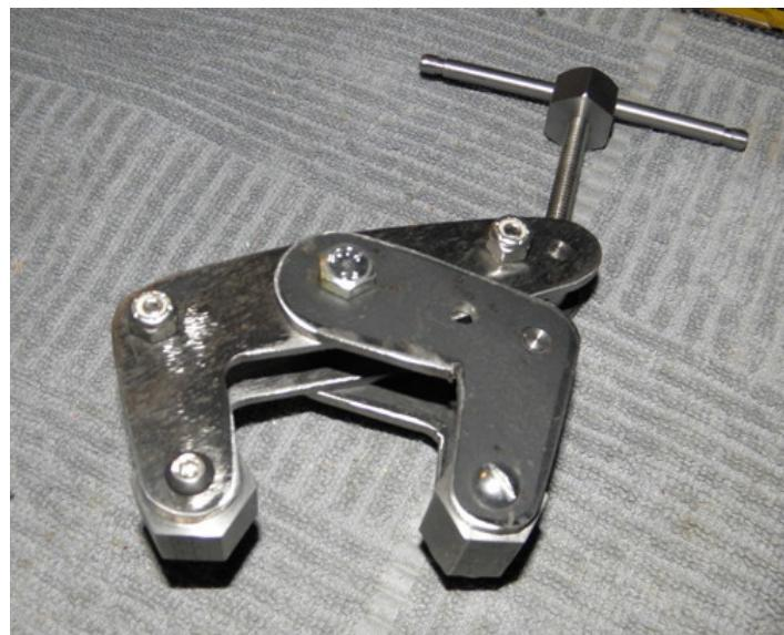
Homemade Kant twist clamp constructed from steel plate, threaded rod, set screws, and screws.
