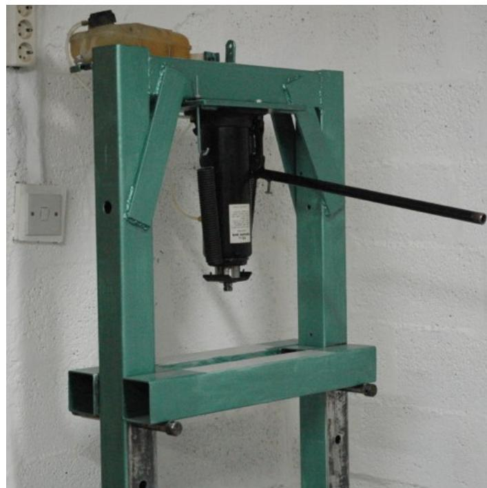
Homemade workshop press constructed from tubing, bar stock, and an inverted hydraulic jack.
