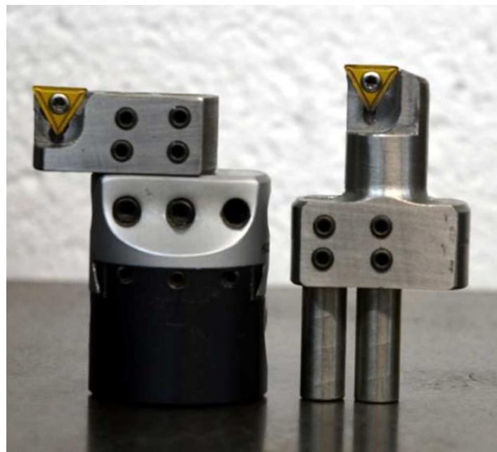
Homemade boring head modification constructed from steel stock and set screws.
