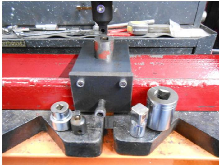
Homemade square hole punch press constructed from sockets and socket adaptors.
