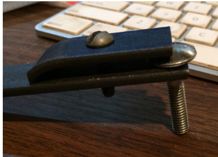
Homemade tee nut jig constructed from bar stock and a screw.
