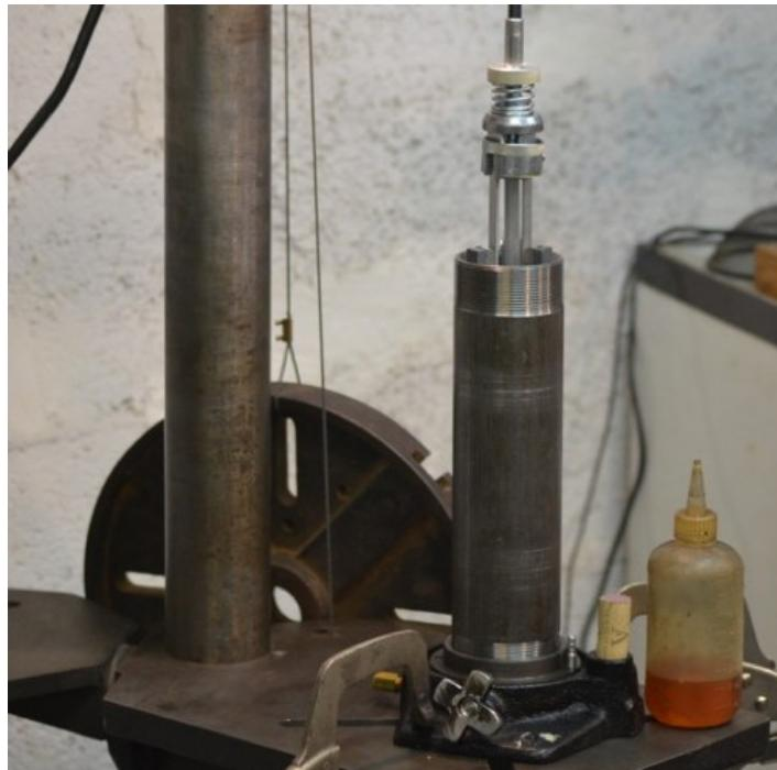
Homemade cylinder honing setup constructed from a drill press and clamps.
