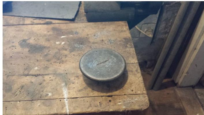
Homemade anvil constructed from a surplus ship engine exhaust valve.
