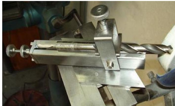
Homemade drill sharpening jig constructed from square and round bar stock, steel plate, washers, and Allen bolts.
