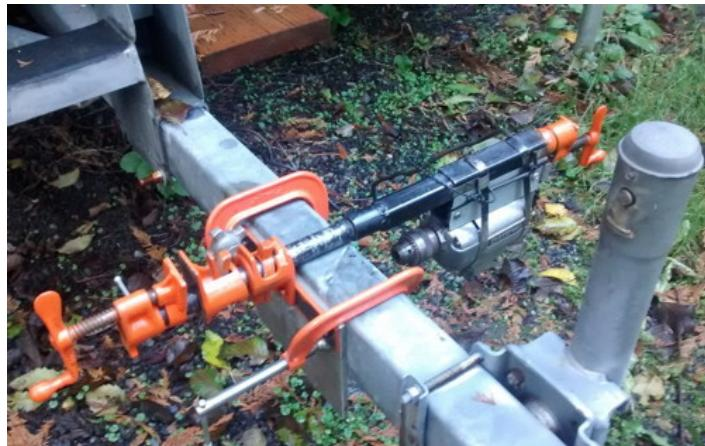
Homemade portable drill press constructed from a surplus drill, pipe clamps, tubing, clamps, and aluminum plate.
