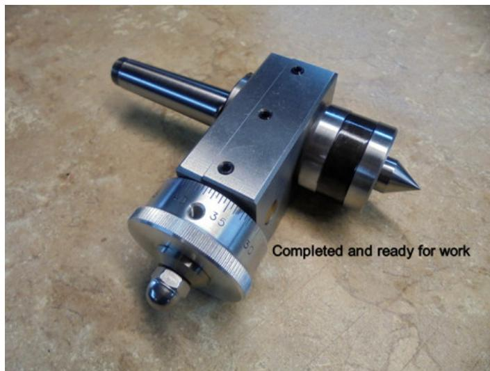
Homemade tailstock taper turning attachment constructed from brass, aluminum and alloy steels. Uses an off-the-shelf Morse taper shank.
