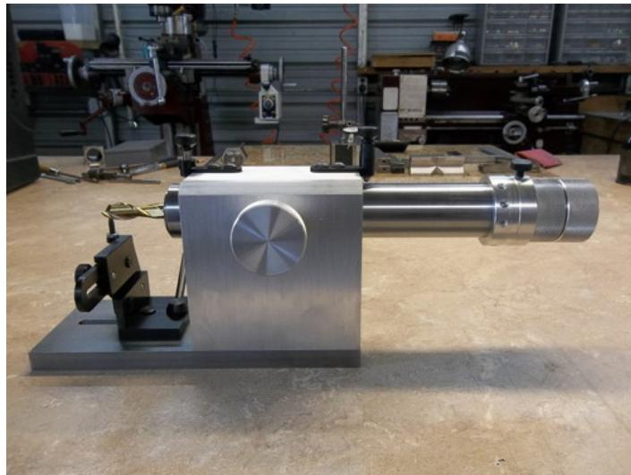
Homemade end mill sharpening fixture constructed from 1018 and O-1 steels, 1020 D.O.M. tubing, and 6061 aluminum.
