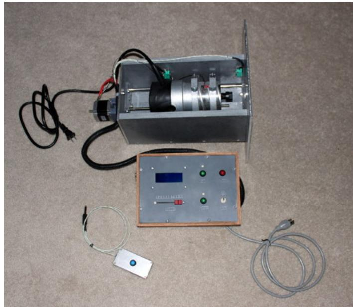
Homemade Arduino router lift constructed from a stepper motor, auto zero probe, an Arduino, and LCD display.
