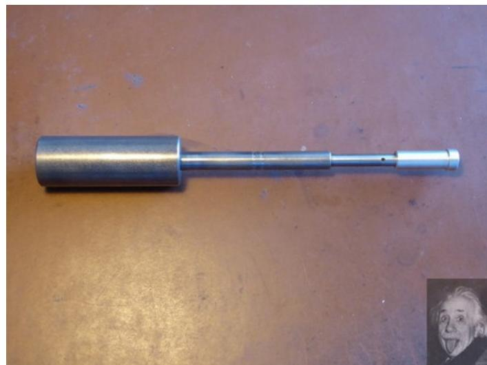
Homemade slide hammer center punch constructed from round bar stock, aluminum, and a set screw.
