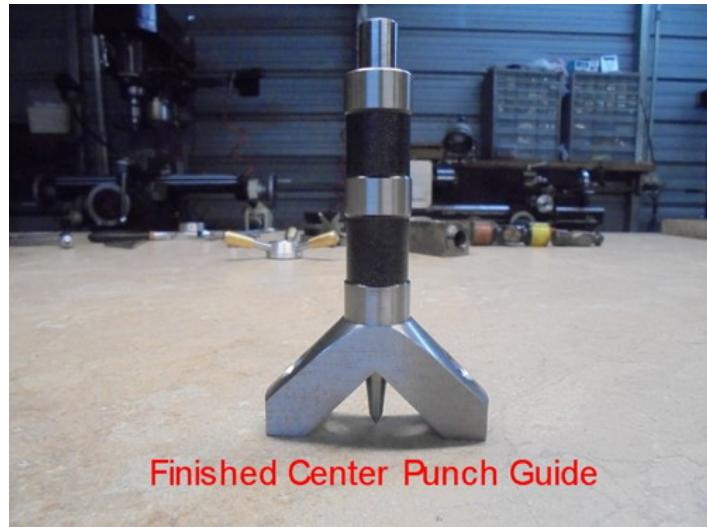
Homemade center punch and guide constructed from 1018 CRS and O-1 tool steel.
