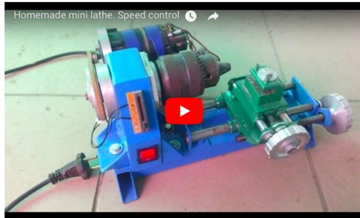
Homemade mini lathe constructed from rectangular tubing, angle iron, a drill chuck, sewing machine motor, and homemade pulleys.
