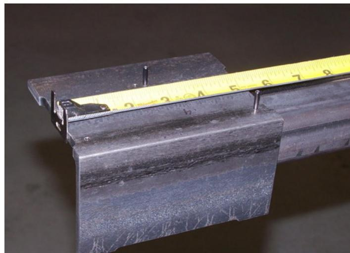
Homemade miter measuring aid constructed from surplus angle iron and pins.
