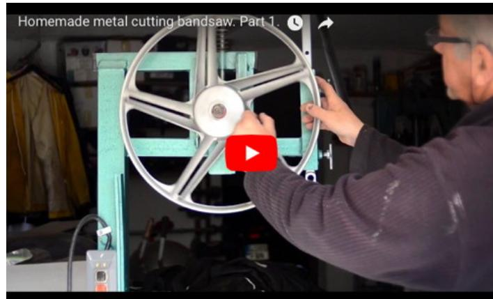
Homemade vertical bandsaw constructed from tubing, bar stock, bearings, a gearbox, electric motor, and moped wheels.
