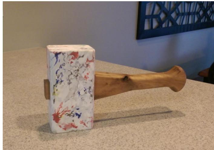
Homemade milk jug hammer featuring a head molded from surplus HDPE. Mounted to a handle fashioned from shipping pallet wood.
