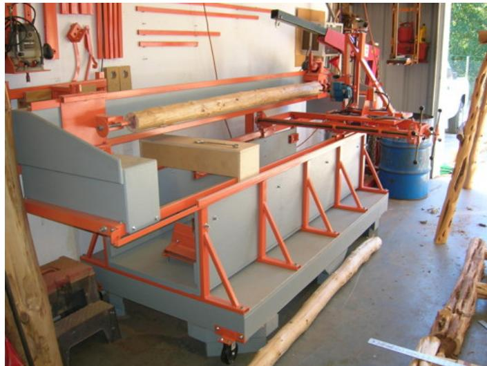
Homemade sawmill constructed from tubing, bar stock, bearings, and an electric motor. Doubles as a lathe, mortise machine, and drill press.
