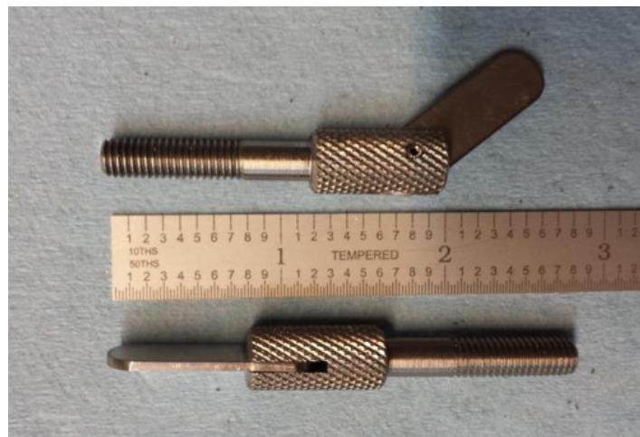
Homemade lever action clamping screws constructed from 1018 CRS rod, roll pins, and surplus steel support rails.
