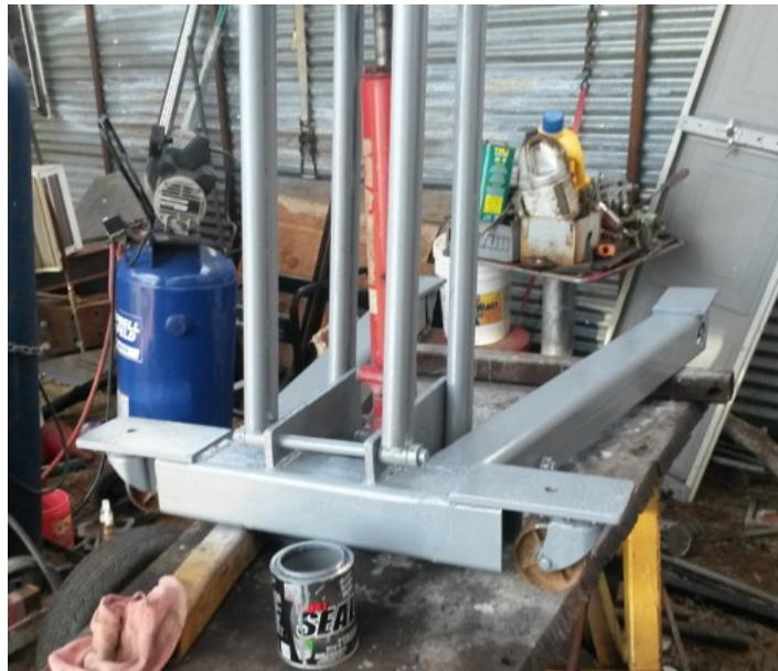
Homemade heavy duty transmission jack constructed from 4x4 square tubing, 1" sprinkler pipe, casters, swivels, CRS bar stock, homemade collars, and a chromed cylinder.
