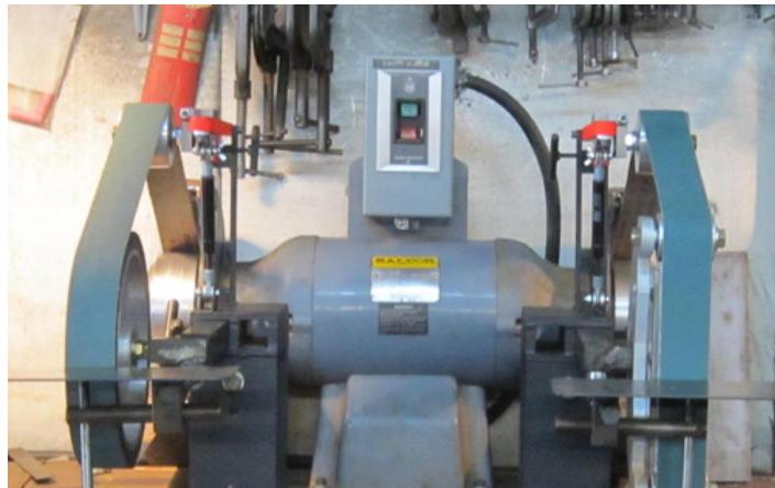
Homemade dual belt grinder and sander constructed from a surplus grinder, steel plate, and grinding wheel.
