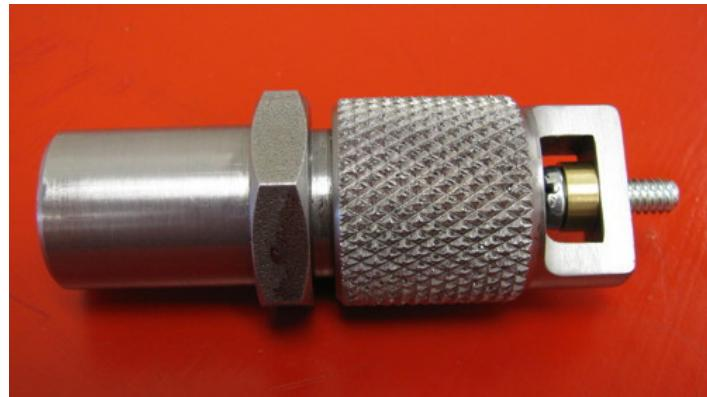
Homemade lantern chuck constructed from 1018 cold rolled steel and brass stock.
