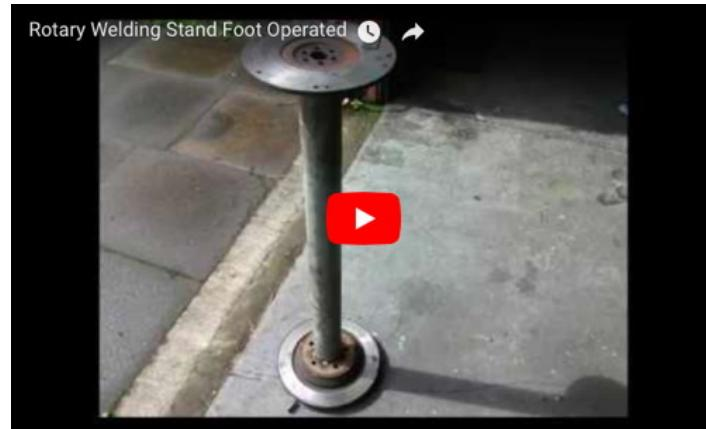
Homemade rotary welding stand constructed from disc rotors, a flywheel, and pipe.
