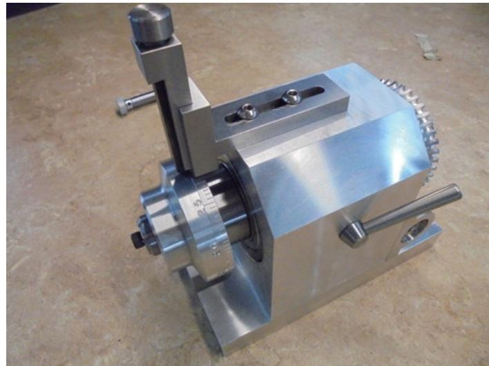
Homemade dial making fixture constructed from steel stock and bearings.
