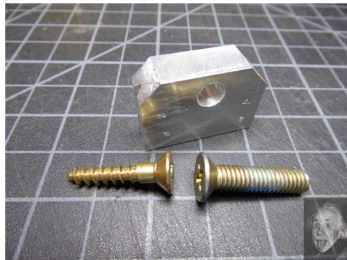
Homemade countersink gage constructed from aluminum stock.
