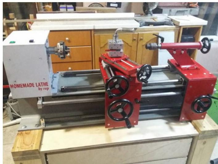
Homemade lathe constructed from a surplus steel beam, lumber, leadscrews, steel plate, and bearings.
