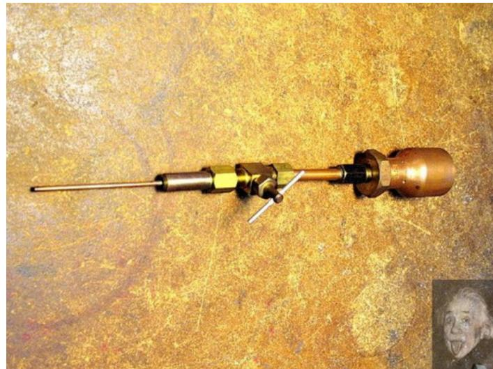
Homemade parting-off oiler constructed from plumbing fittings, scrap tubing, and a valve.
