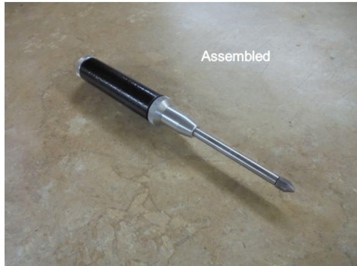
Homemade oil injector constructed from bar stock, tubing, a nozzle, and O-rings.
