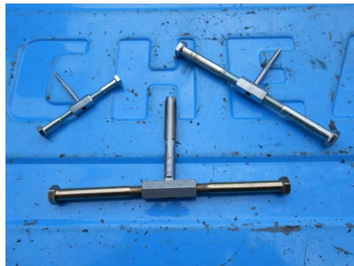
Homemade tap holders constructed from coupling nuts and bolts.
