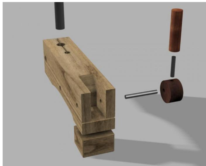
Homemade quick clamp constructed from surplus oak and steel pins. Used for clamping workpieces on a mitre saw.
