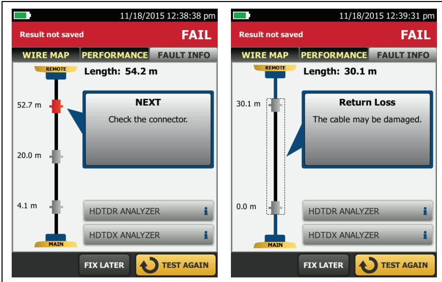
Figure 36. Examples of Fault Information Screens
