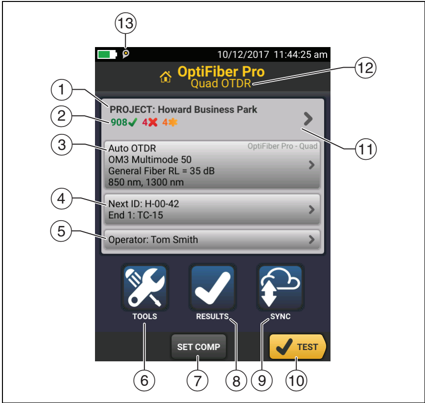
Figure 139. The HOME Screen for OptiFiber Pro Modules
