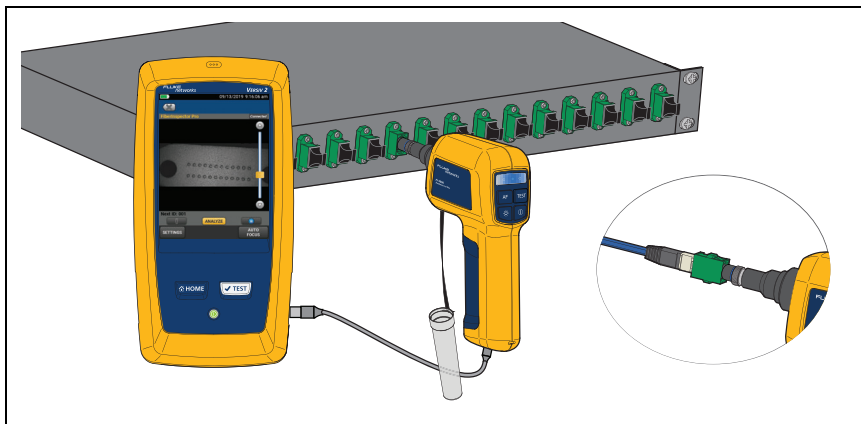
Figure 107. Inspect an Endface (FI-3000 shown)
