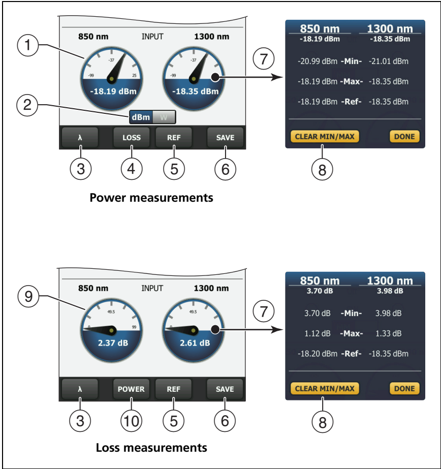
Figure 135. Power Meter Measurements and Controls
