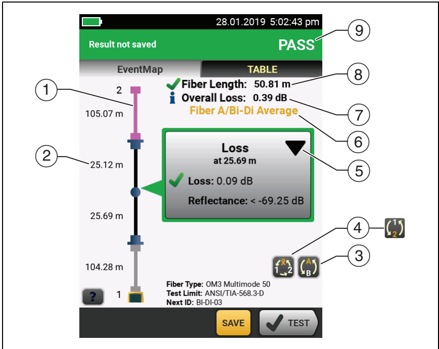
Figure 167. EventMap for Averaged, Bi-directional SmartLoop Results
