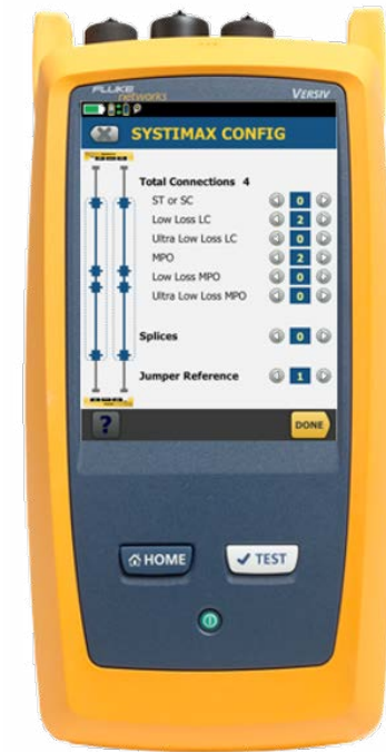
Figure 17 – The CertiFiber® Pro highlighting the SYSTIMAX Fiber Performance Calculator
