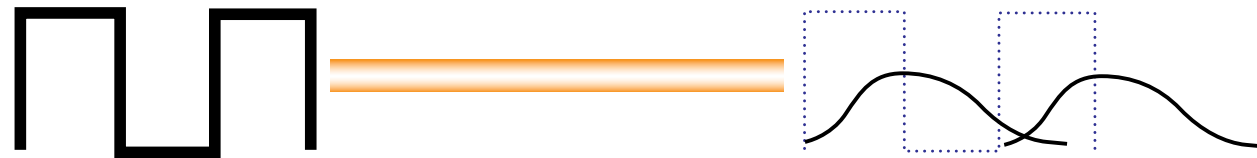
Figure 9 – The net effect of dispersion causes the transmitted pulses to run together and overlap at the end of the link (input to the detector). The detector can no longer recognize and decode the state of individual pulses.
