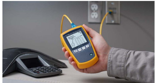
Figure 5. The MicroScanner PoE can detect the power offered by the PSE plus the network's speed, and features a suite of cable testing features.
