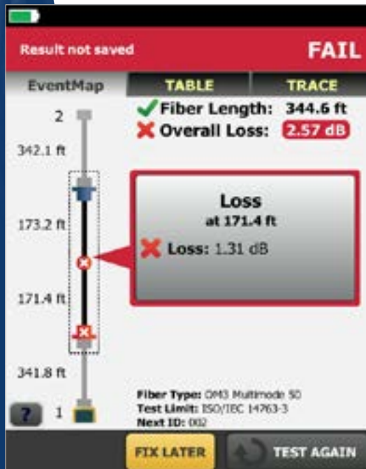
Figure 41. OptiFiber Pro EventMap identified a FAIL
