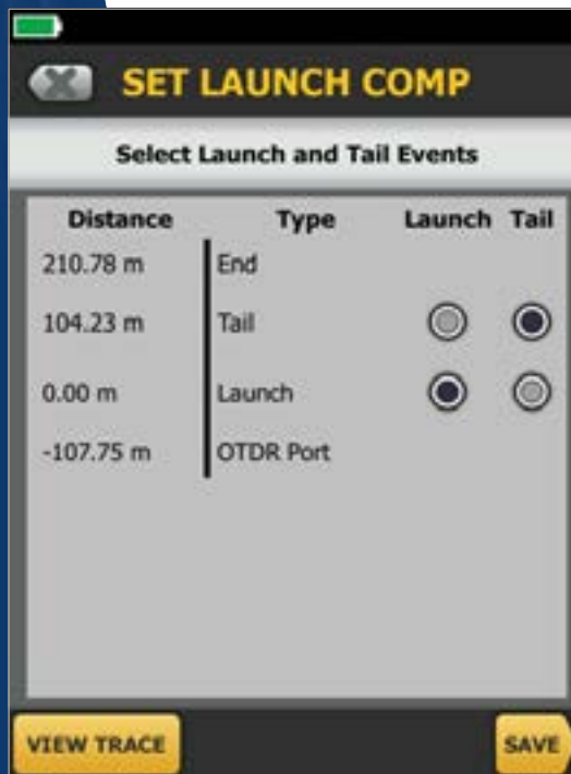
Figure 32. Set Launch Compensation results screen
