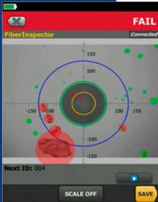
Figure 3. Fluke Networks FI-7000 FiberInspector™ Pro “FAIL” screen
