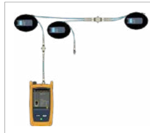
Figure 31. SmartLoop launch fiber compensation setup
