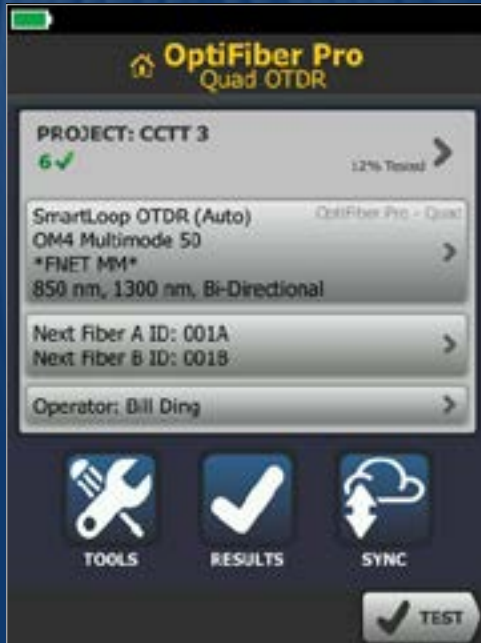
Figure 25. OptiFiber Pro with a multimode test set up
