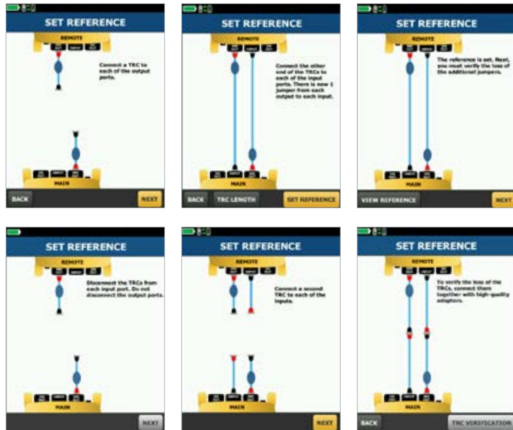
Figure 15. Set Reference Wizard showing how to set the reference on the EF compliant TRCs and measure the loss of the patch cords you will add.
