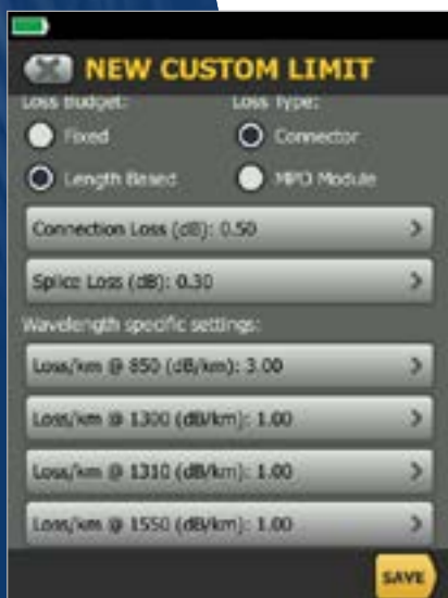
Figure 13. CertiFiber Pro Customs limits setup screen.
