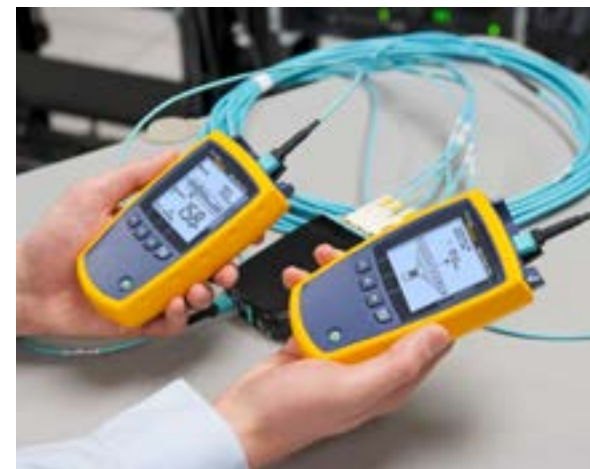
Figure 20. MultiFiber Pro making MPO testing easier and faster
