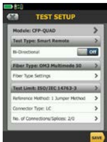
Figure 11. Test setup for Test Type, Fiber Type and Test Limit
