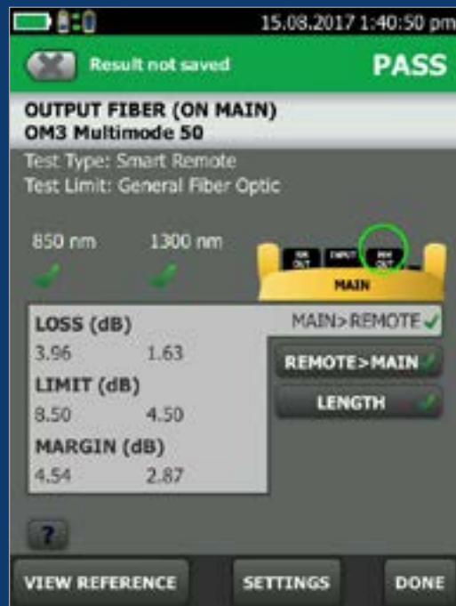
Figure 18. Results of CertiFiber Pro Bi-directional OLTS test
