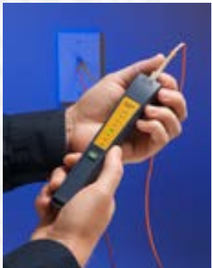
Figure 40. SimpliFiber Pro FindFinder helps identify cable IDs.
