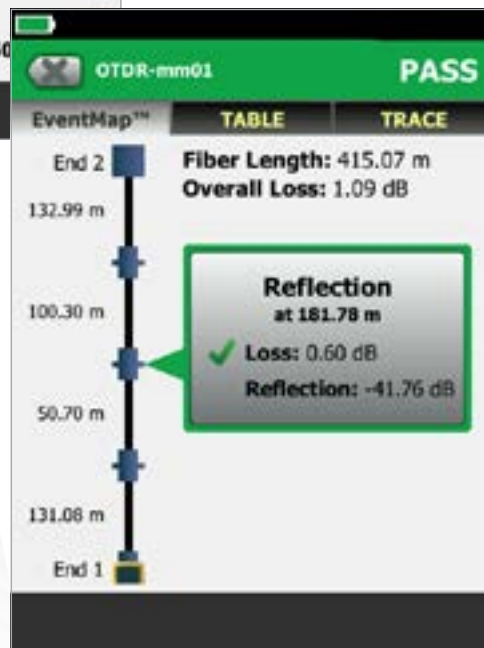
Figure 23. OptiFiber Pro EventMap™ example
