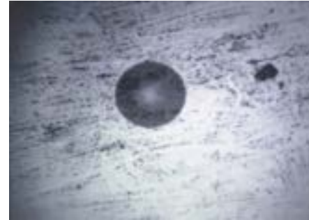
Figure 5. Contaminated fiber end-face
