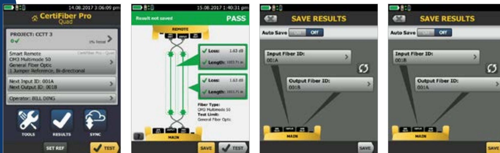
Figure 17. CertiFiber Pro OLTS screens from a bi-directional test
