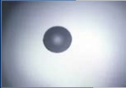
Figure 6. Clean fiber end-face
