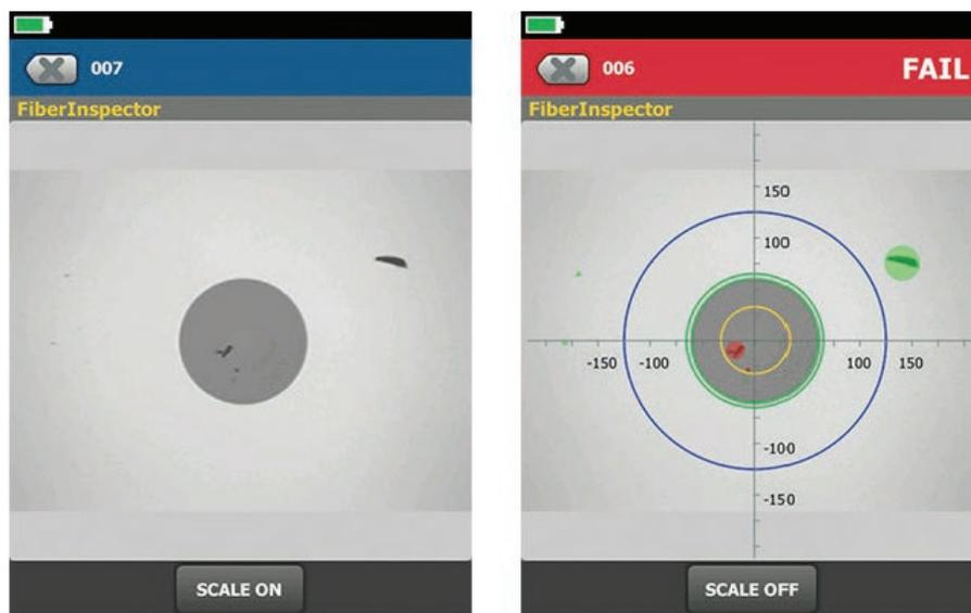
Figure 5: Is the endface shown on the left clean or dirty? Automated certification demonstrates that it is dirty per IEC 61300-3-35 due to defects in the core.
