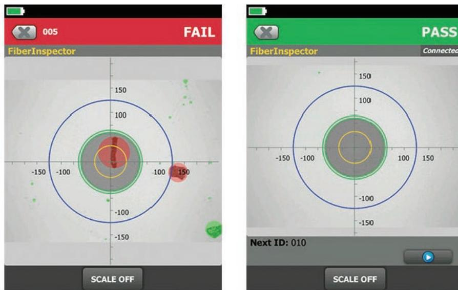
Figure 10: The FI-7000's certification results allow you to quickly determine if the fiber endface pass or fails. An example of a failing endface is shown on the left and a passing endface is shown on the right.
