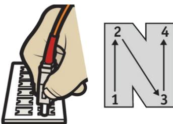
Figure 8: “Wet to Dry”: cleaning methodology Using a Fluke Networks Optic cleaning card. The solvent drop is placed at “1”, and the end face moved across the cleaning material from “1” to “4”
