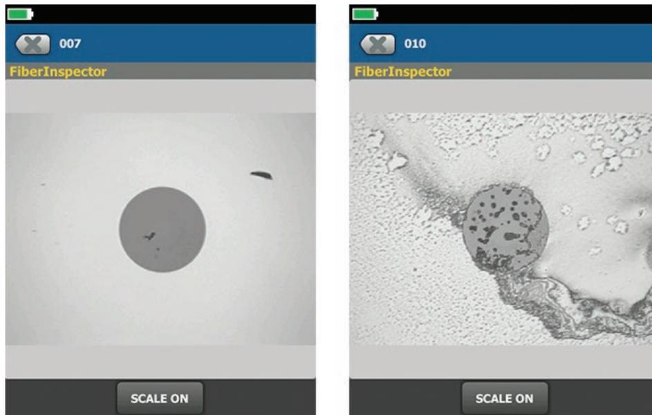
Figure 9: Specialized solvents (left) are far more effective at cleaning endfaces than IPA that can leave behind a residue (right).
