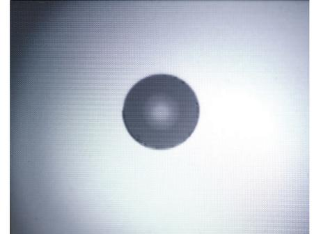
Figure 6: Clean fiber end-face.
