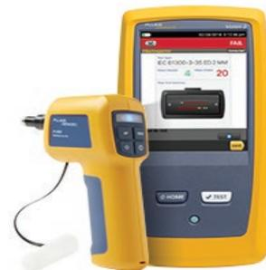
Figure 2c: Fluke Networks FI-7300 FiberInspector Pro MPO / Single fiber inspection camera provides automated PASS/FAIL results and uses Versiv for display, user interface and recording of results.
