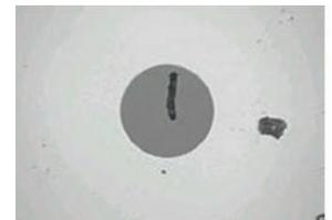
*Figure 1: Dirty fiber endfaces as shown here can degrade network performance or damage equipment*
