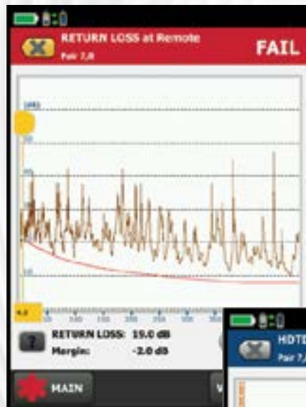
Figure 7. Return loss failure with worst pair 7/8 reporting -2.0 dB margin @ 4.9 MHz
