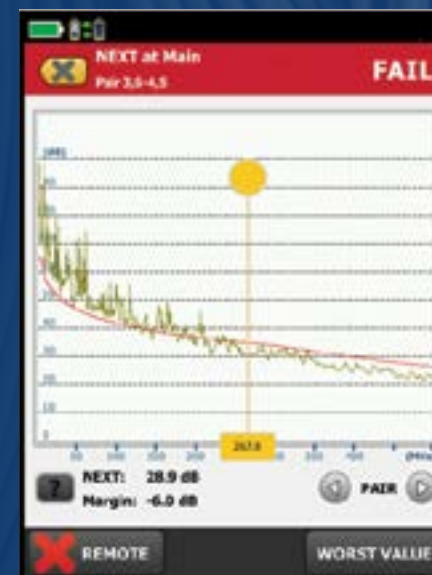
Figure 13. Next failure at -6.0 dB Margin @ 267.0 MHz on Pair 3,6 -4,5
