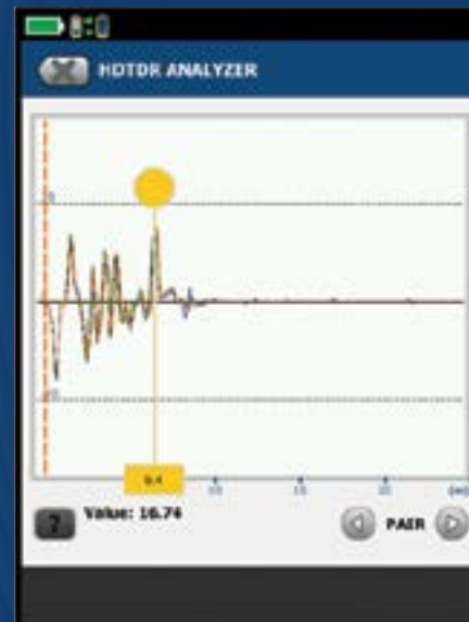
Figure 10. The HTDR analysis shows Return Loss at the beginning of the cable for all four pairs, usually a characteristic of water in the cable
