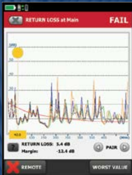
Figure 9. Return Loss failures on all pairs at the low frequencies
