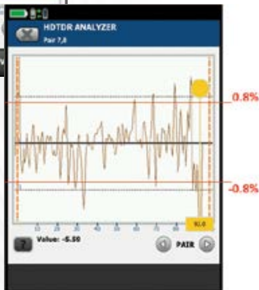
Figure 8. HTDR showing Return loss issues along the whole cable
