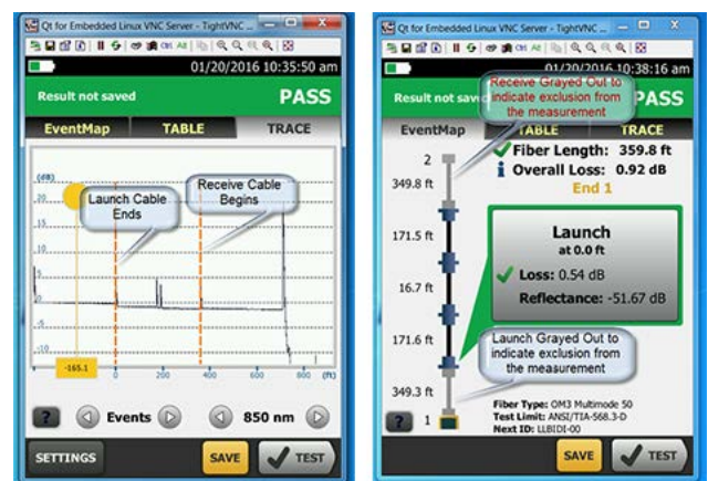
Figure 4. The trace includes the launch and receive fibers at the beginning and end of the link under test. The EventMap shown at right uses launch compensation to remove their effects from the test results.
