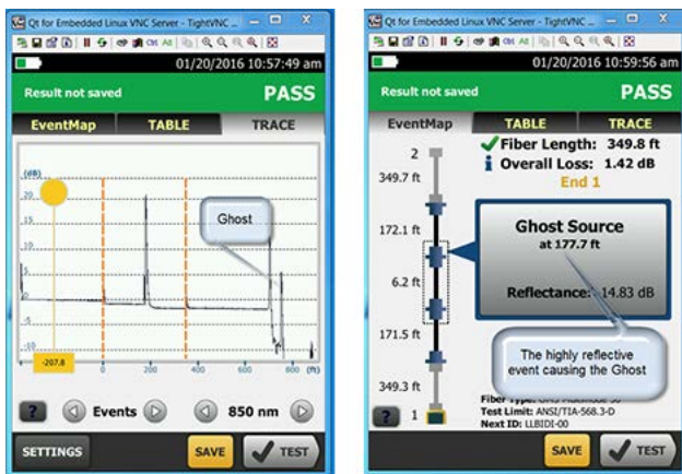
Figure 9. “Ghosts” are non-existent events resulting from strong reflected signals from actual events.
