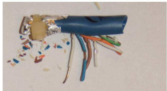
Fig. 2 Cable damage and insulation degradation after 10 days at 120 degrees C.
