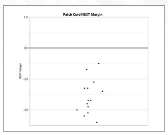
Figure 8: Patch cords from channels in figure 6 measured by CommScope
