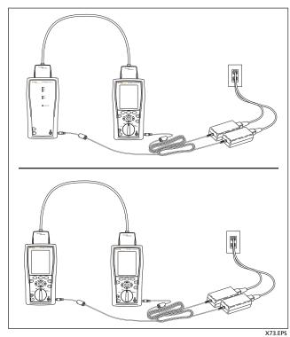
Figure 23. Updating the Software with an Updated Tester
