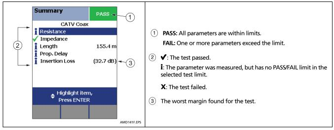
Figure 21. Autotest Results for Coaxial Cabling
