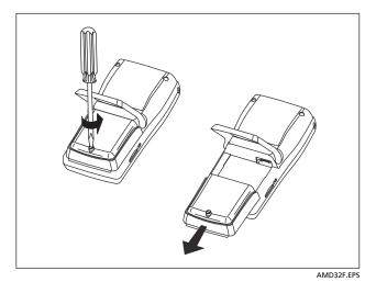
Figure 4. Removing the Battery Pack
