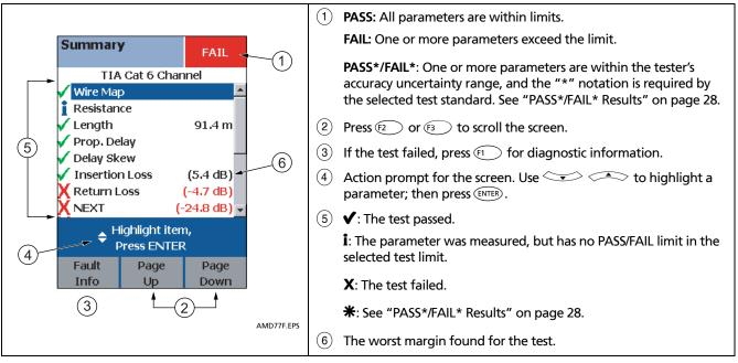
Figure 14. Autotest Summary for Twisted Pair Cabling
