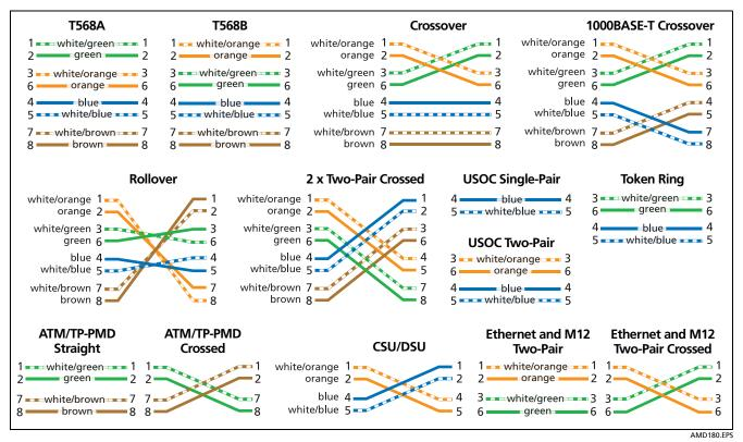
Figure 10. Outlet Configurations
