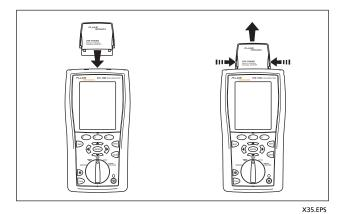
Figure 6. Attaching and Removing Adapters
