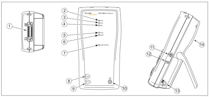
**Figure 3. Smart Remote Features**
