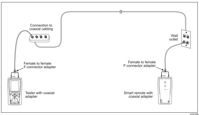
**Figure 20. Coaxial Video Cabling Test Connections**
