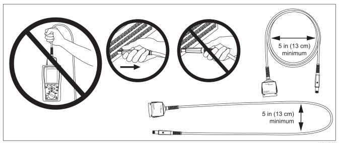
Figure 7. Handling Guidelines for Optional Permanent Link Adapters
