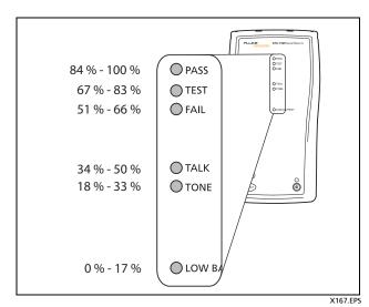
Figure 5. Smart Remote Battery Status Shown After Power-Up
