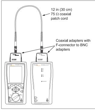
Figure 17. Coaxial Reference Connections
