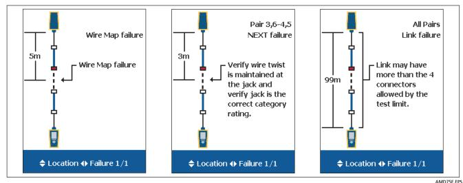
Figure 16. Examples of Automatic Diagnostic Screens
