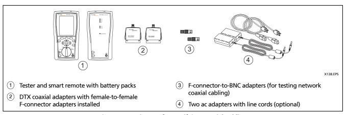
Figure 18. Equipment for Certifying Coaxial Cabling
