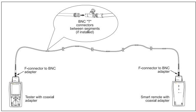
**Figure 19. Coaxial Network Cabling Test Connections**
