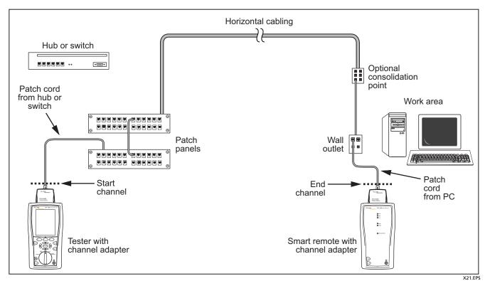
**Figure 13. Channel Test Connections**
