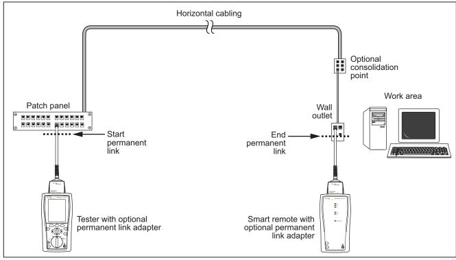
Figure 12. Permanent Link Test Connections
