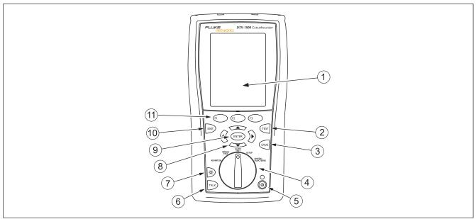
**Figure 1. Tester Front Panel Features**
