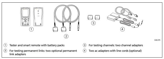
Figure 11. Equipment for Certifying Twisted Pair Cabling
