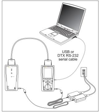
Figure 22. Updating the Software with a PC
