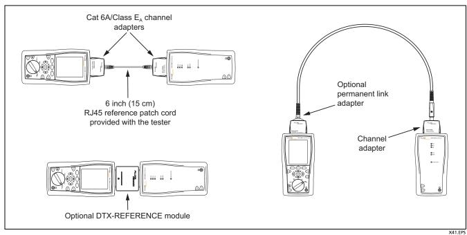
**Figure 9. Twisted Pair Reference Connections**
