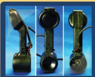
Rotary test sets emerge for line verification testing.
