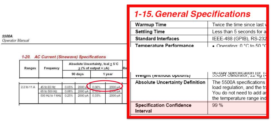
The manufacturer's specs document that specifications are based on a normally distributed, 99% confidence interval
