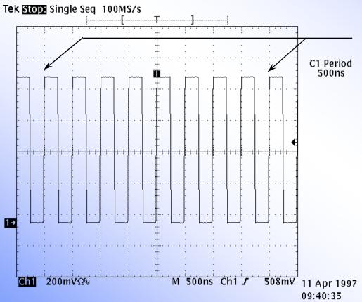
2<sup>nd</sup> and 10<sup>th</sup> rising edges aligned with according graticule lines
