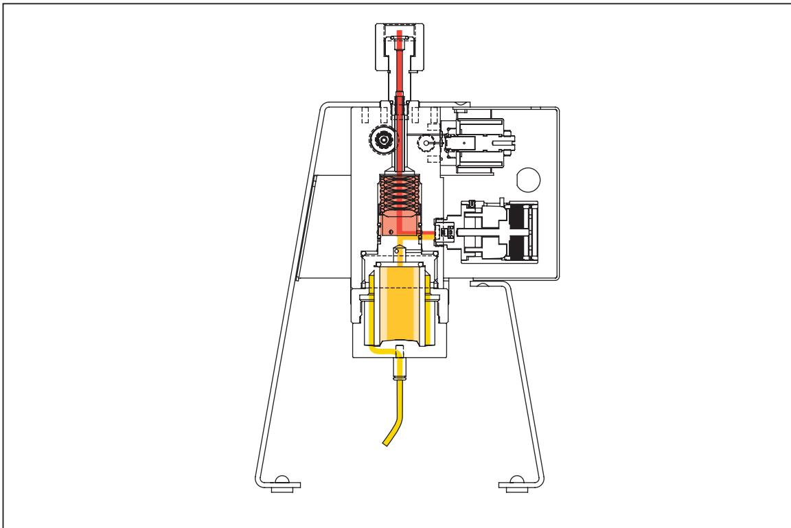
**Figure 2. Cutaway of the CPS-40M-HC40 during a Normal Downward Pressure Excursion, or Purge Task**
