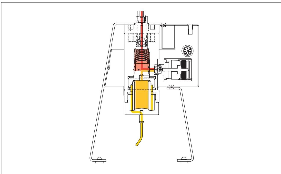
**Figure 3. Cutaway of the CPS-100M Purge Task during a Normal Downward Pressure Excursion, or Purge Task**
