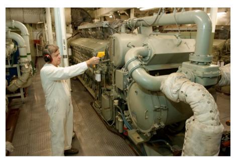
The ferries in Washington State transport over 24 million people per year. They are propelled by 3.5 megawatt, 4160-volt motors. The maintenance staff uses a wide array of Fluke industrial test tools to measure the voltage, current and temperature of the propulsion system.
