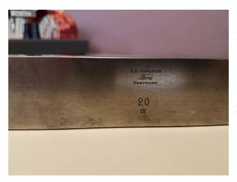
For example, the second industrial revolution, known as the technological revolution, was enabled by developing methods for interchangeable parts. Henry Ford became one of the key players in this revolution by building automobiles on an assembly line. This would not have been possible without routine calibration. Here is an antique length standard used for calibrations during this time. It was manufactured by a joint venture between Ford and C.E. Johanssen, the inventor of the gage block.
