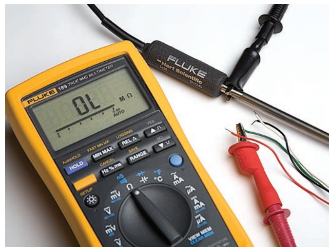
Using a Fluke 189 DMM, one lead is clipped to one of the probe leads, and the other lead is clipped to the sheath near the handle. The 189 indicates "OL" on the Ohms Range at room temperature. This signifies an insulation resistance greater than 500 MΩ and is considered good.
