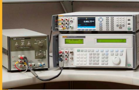
Since the 1960's, commercial voltage and ratio calibration systems have been available to calibrate dc voltage from very low levels—on the order of millivolts—to relatively high values up to 1 kilovolt. A critical component of these systems was the analog high impedance voltmeter/null meter. These instruments were designed with extremely high input impedance (10 to 100 M $\Omega$ ), excellent sensitivity (0.1  $\mu v$  per division) and high isolation (on the order of  $10^{12} \Omega$ ).
