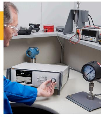
pressure is unstable. Changes in pressure must align with one or more of the three variables: volume change (expansion or contraction of pressure lines); change in number of molecules (a leak); or temperature effects (as the temperature of the fluid cools, the pressure decreases with it).
