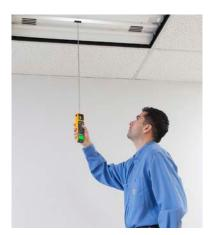
The Fluke 1000FLT Fluorescent Light Tester takes the trial and error out of fluorescent light testing. It is the only tester that performs all five essential lighting tests in less than 30 seconds. For people who work with large numbers of fluorescent lights, the Fluke 1000FLT is an indispensable trouble shooting tool.
