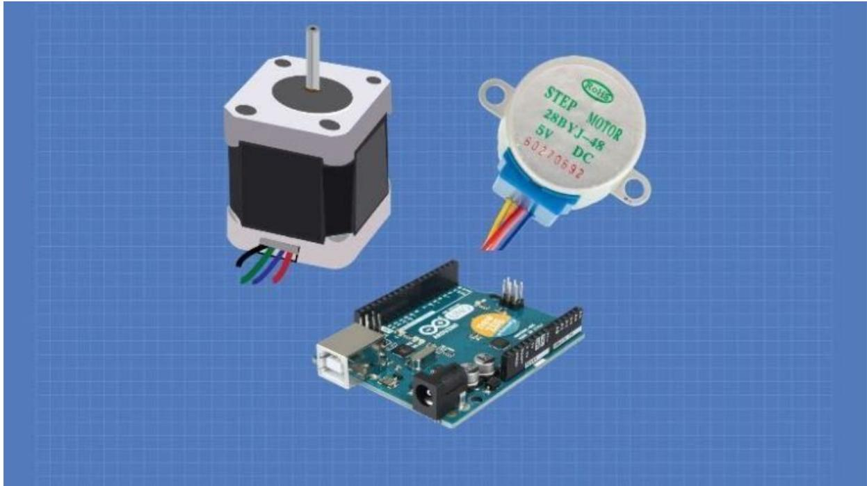
Unlike DC motors stepper motors are controlled by applying pulses of DC electricity to their internal coils. Each pulse advances the motor by one step or by a fraction of a step, the latter is known as “microstepping” and will be explained shortly.
