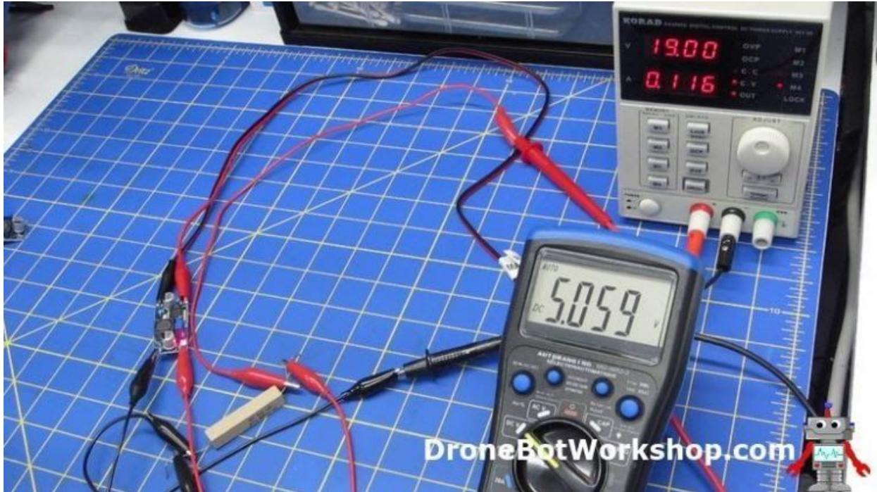
I then switched to the “fixed” converter and turned the multi-turn potentiometer so that it gave an output of 5-volts.
