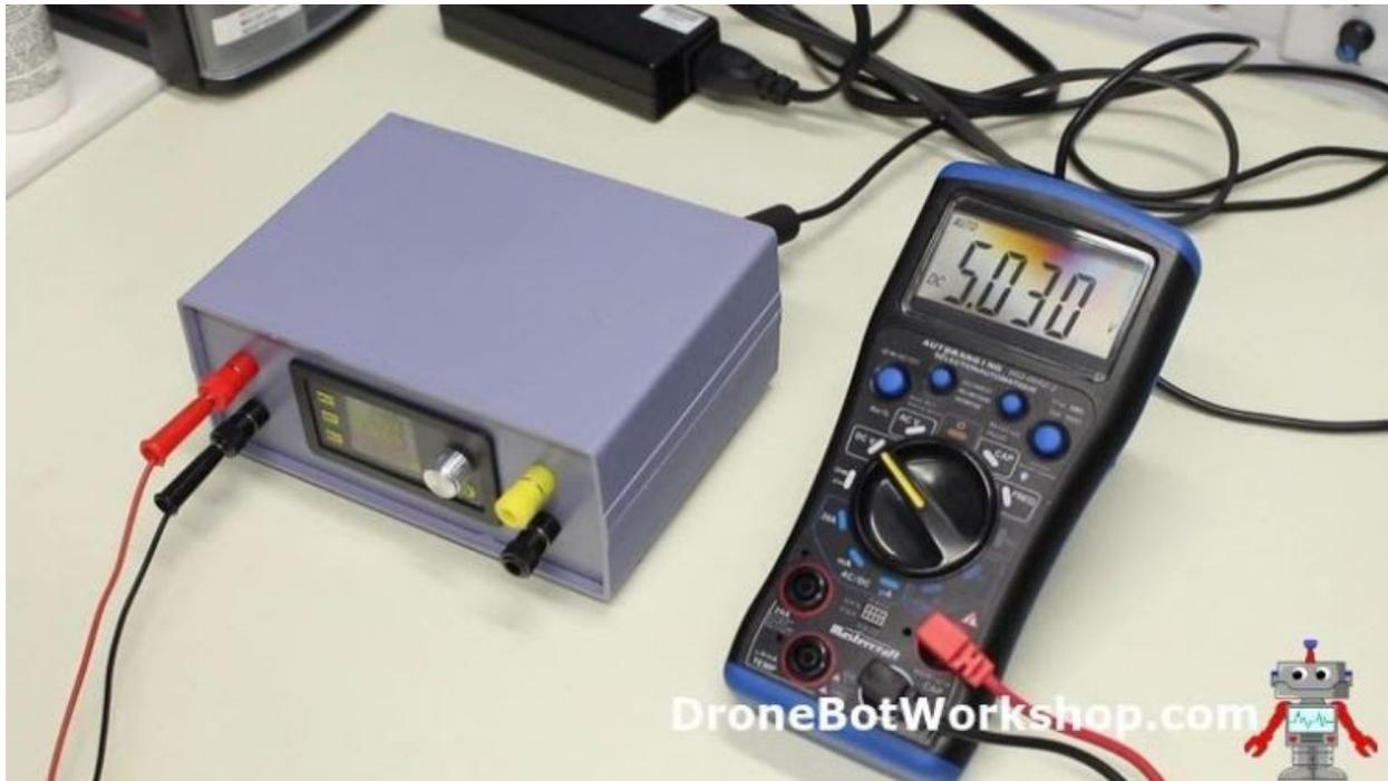
Get the same test load you use before and hook it up to the 5-volt output, along with your multimeter in voltage mode. Adjust the multi-turn potentiometer on the fixed module to obtain as close to 5-volts as you can.
