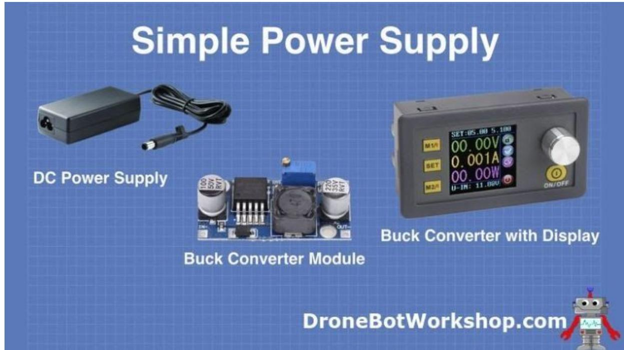
Here are the parts that I used in my simple power supply design.
