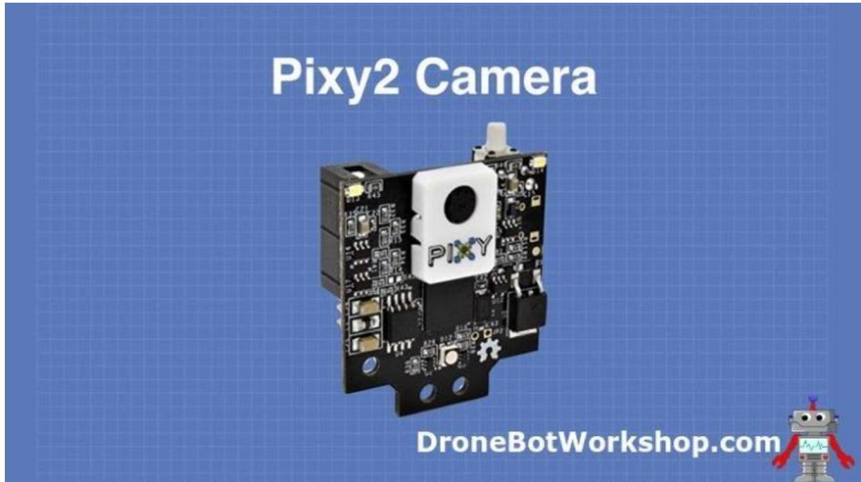
The Pixy2 is capable of recognizing seven distinct objects based upon their shape and color (or hue). Each of these objects is assigned a unique “signature”.
