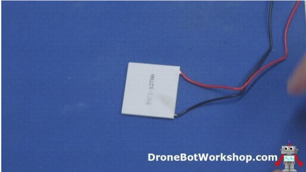
The module has two leads, a red one and a black one. These are for powering it, I used a 12-volt power supply for my module. As Peltier modules are not very efficient you'll need a good amount of current to drive this, I recommend using a power supply capable of 6 amperes.
