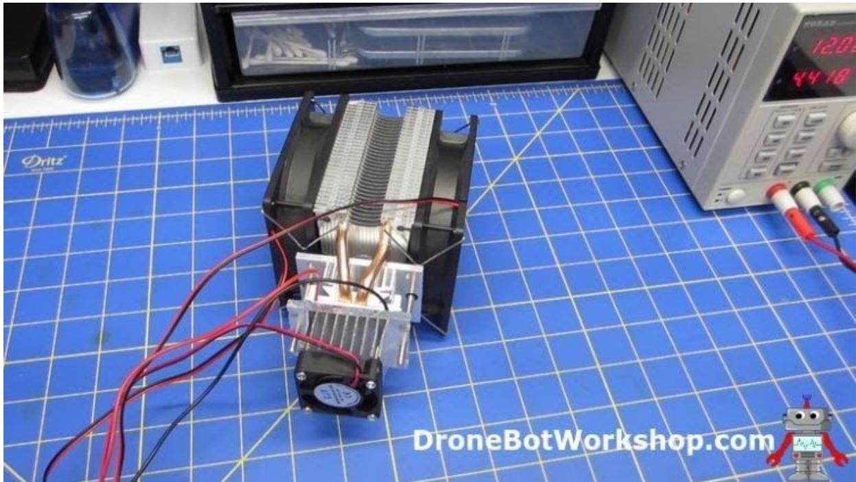
If nothing else these assemblies are a great source of parts for a very low price. The one I obtained had three fans, a Peltier module, and several heatsinks and heat pipes. It even came with a new 12-volt 6-ampere power supply. A great deal when you consider it costs about as much as the power supply would by itself!
