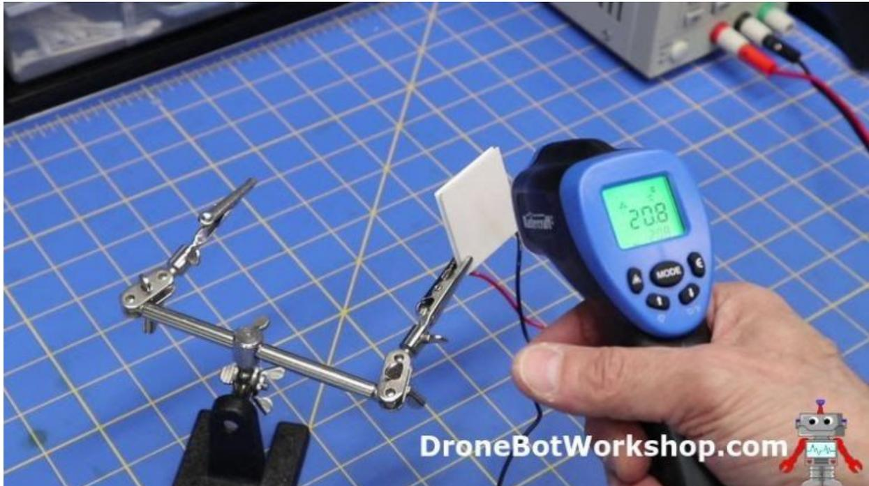
In my case, it measured 20.8 Celcius, which is about right for the ambient temperature in the workshop when I made the measurements.
