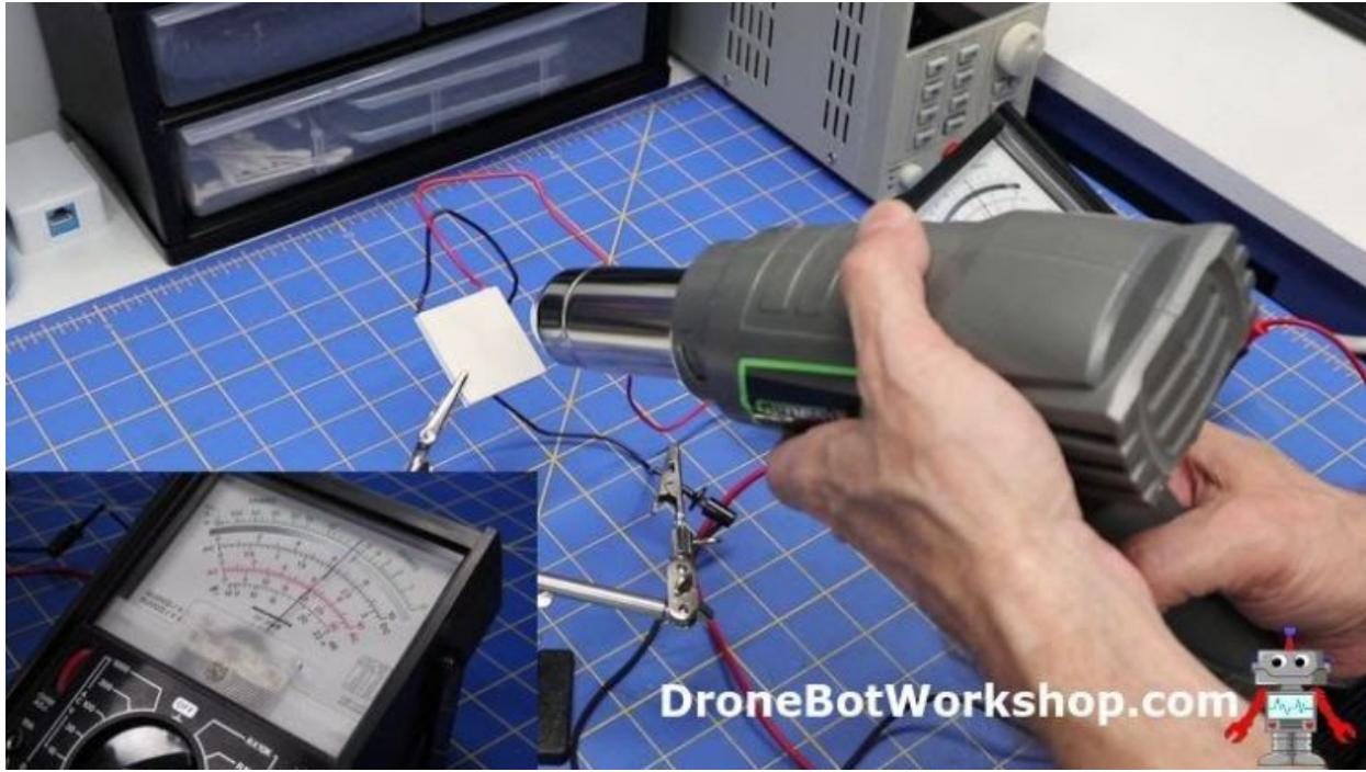
I managed to obtain about 1.5 volts from my module after I heated it up. Not enough to really do anything with, especially as I suspect it was very low-current.
