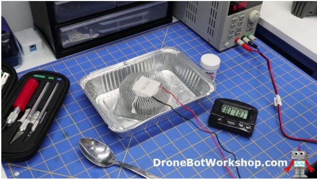
I applied power to the Peltier module and observed that it immediately started getting cold. I then took a couple of drops of water and placed it on top of the module.
