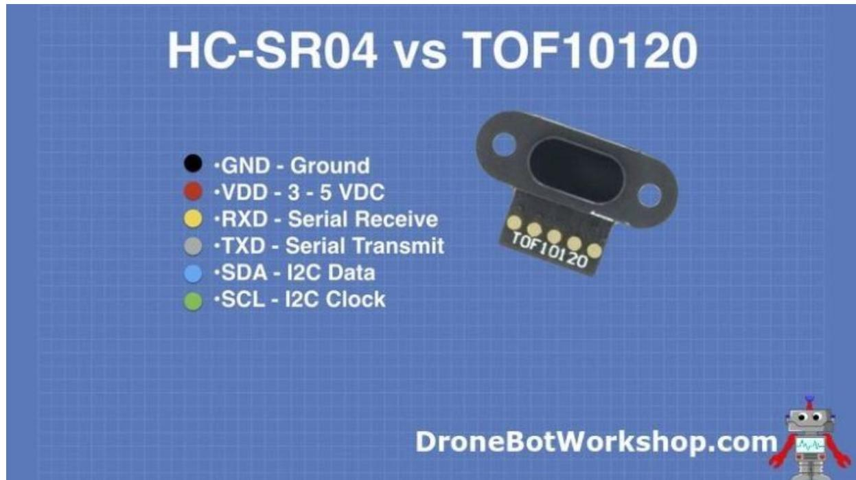
The device operates on voltages between 3 and 5-volts, so it is suitable for use with 3.3-volt logic. It has a stated range of 10 – 180 cm.
