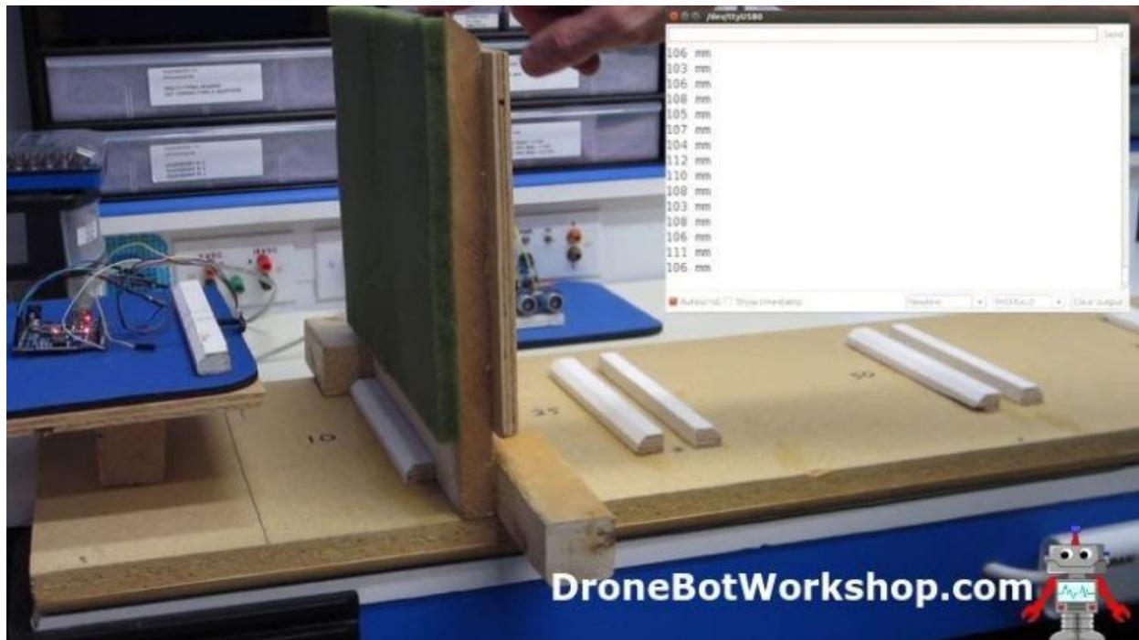
It seems the laser beam passed right through the foam and hit the underlying board. Just as the ultrasonic sound waves did. I hadn't expected that.
