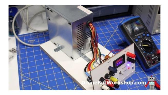
I mounted my supply on a block of wood, along with a terminal strip for breaking out the connections from the ATX supply.
