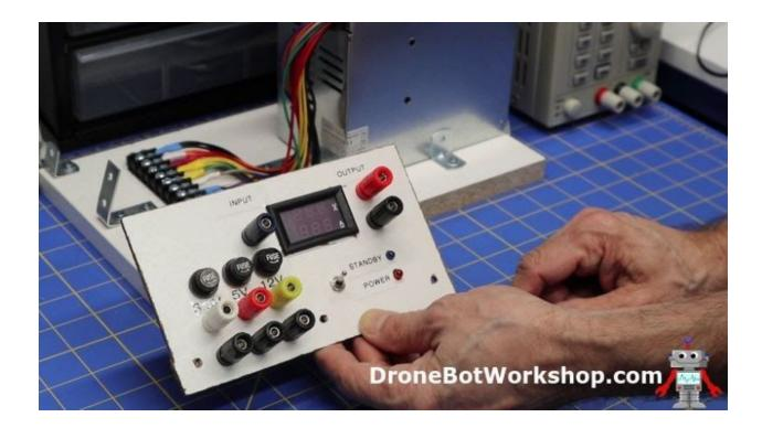
I used lugs on all of the wires to neaten up the hookup. I crimped and soldered the wires to the lugs and covered everything with heat-shrink tubing to keep the connections insulated.
