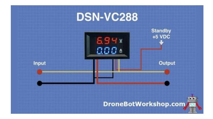
Note that I decided to use the Standby voltage to power the meter, I need to do that because the module requires 4.5 to 30 volts to work and my lowest supply voltage is 3.3-volts.
