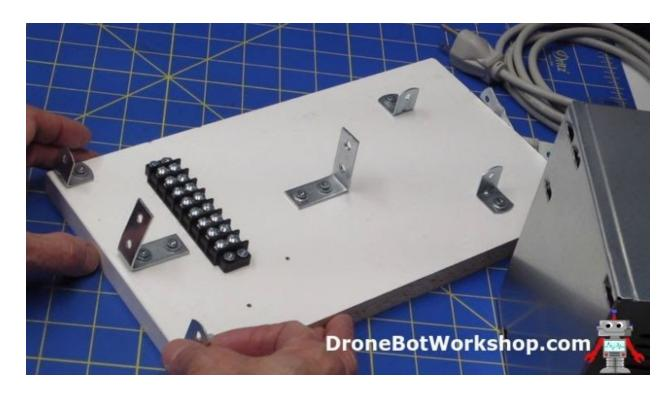
I used the existing threaded screw holes on the back of the ATX supply and a couple of homemade brackets (actually just flattened a couple of small angle brackets in my bench vise) to mount the ATX power supply to the base.
