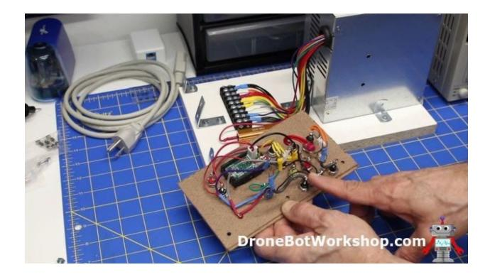
For the power and ground wires I used groups of three wires, this increases the current output capability of the supply (and its the reason there are so many connections on the ATX power supply in the first place). I also have two sets (total six wires) for ground.
