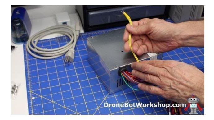
I brought out an additional 5-volt (red) and ground(black) wire to attach to the power resistor that I'm using as a load. If your supply doesn't require a 5-volt load on startup you can eliminate this.
