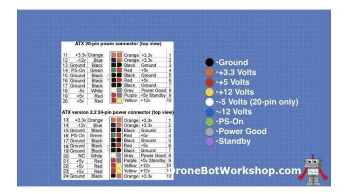
Note that the primary difference is that the 24-pin connector has additional voltage and ground lines.
