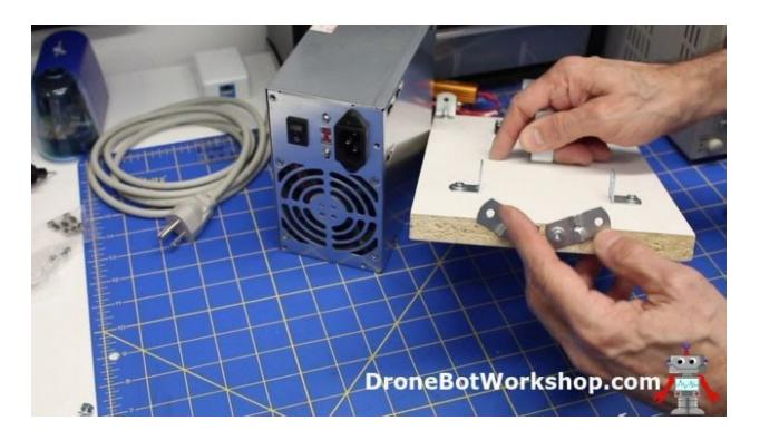
I also constructed a very simple front panel with a thin piece of wood, it's not pretty but it is functional. In addition to the binding posts, switch, fuse holders and LEDs I also mounted a small Voltage and Current meter on my front panel. More on that later.
