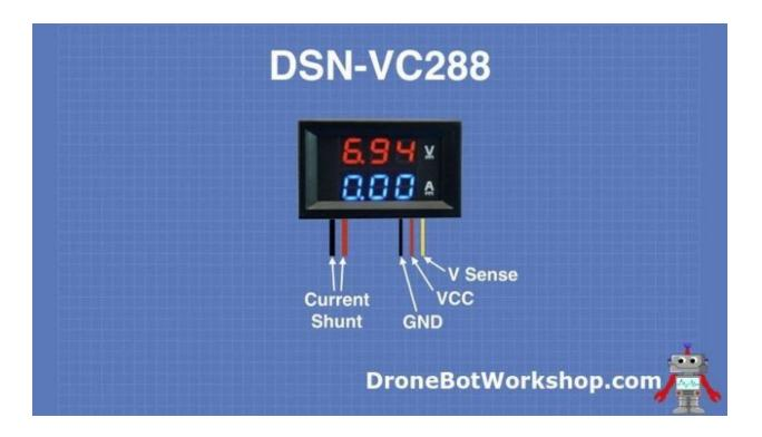
There are two connectors at the bottom of the meter, and it is supplied with cables for each of them.
