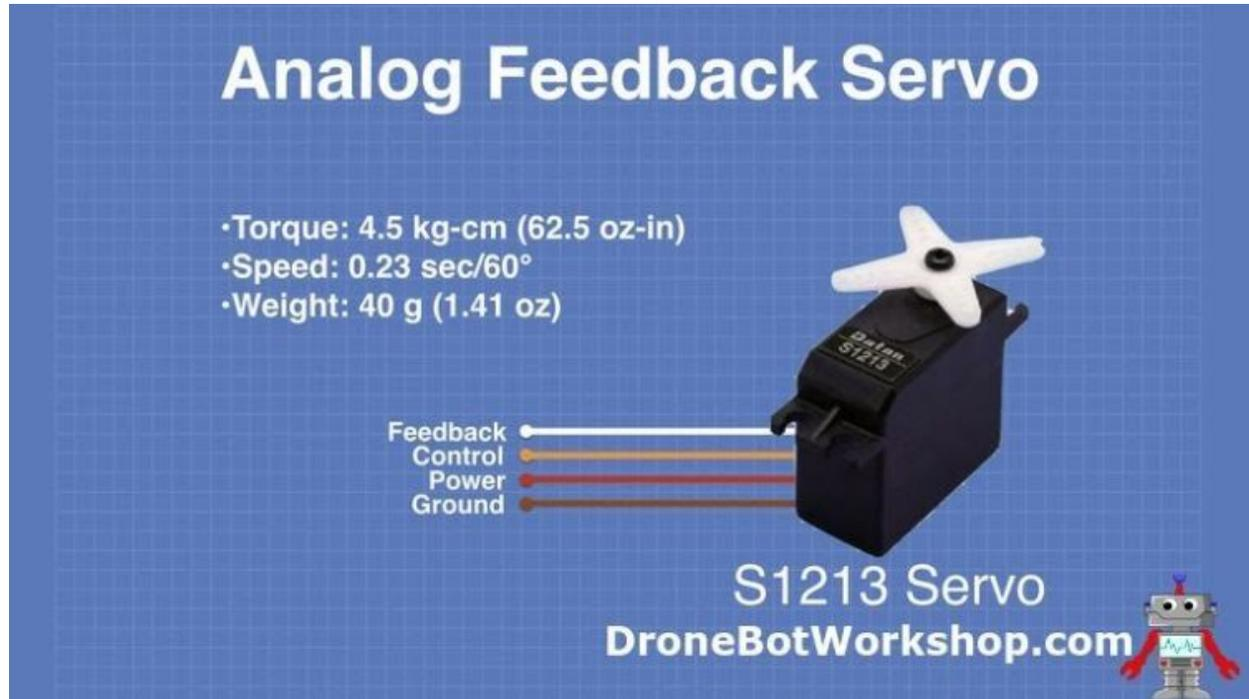
The S1213 is a mid-sized plastic-gear servo motor with an additional feedback output. It operates on 5- VDC and has a torque rating of 4.5 kg-cm, which is robust enough for many applications.
