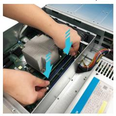
Using two fingers, carefully push down on the memory module until the ejector clips lock it into place.
