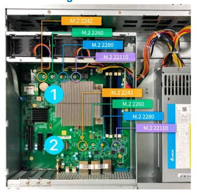
Insert M.2 SSD Drive at a 45° angle and gently push into slot.
