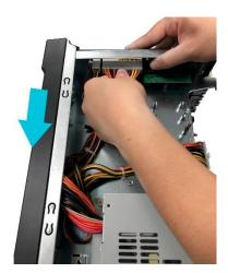
■ Undo M.2 screw and gently lift M.2 assembly from motherboard.
