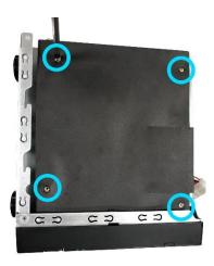
Gently lift motherboard from chassis in the direction as indicated by the arrow.
