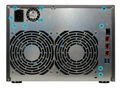
■ Remove case screws on the left and right.
