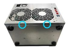
Remove screw holding in backplane and slide left to remove.
