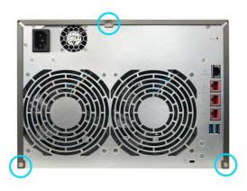
Grip the cover from both sides with two hands and then gently push towards the rear of the NAS to remove it from the chassis.
