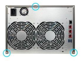
Grip the cover from both sides with two hands and then gently push towards the rear of the NAS to remove it from the chassis.
