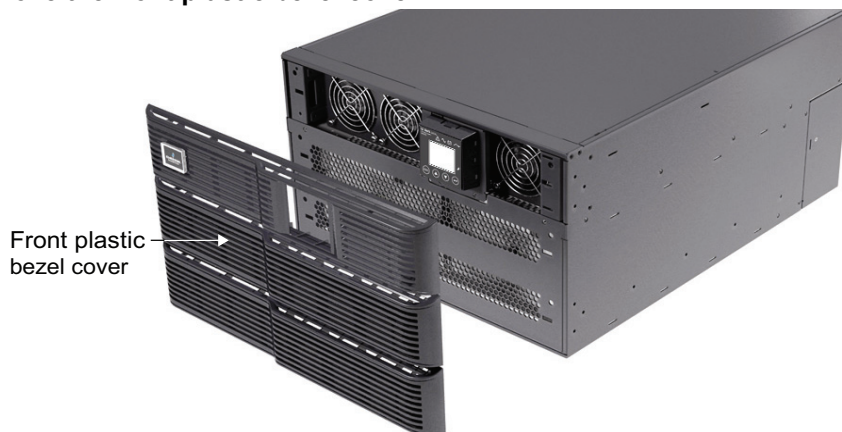
Figure 10 Remove the front plastic bezel cover
