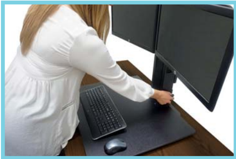
1) Twist knob to loosen
