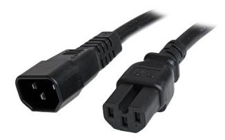
The PXTC14C156 C14 to C15 Power Cord (6 ft) features a C15 connector rated for high-temperature equipment, as well as 14 AWG wire suitable for high power connections - a reliable solution for connecting to C14 Power Distribution Units (PDU) located in switchgear rooms and data center environments, or large server applications that require a higher rated, heavier gauge cable.
