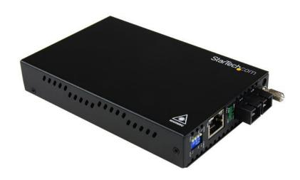
The ET91000SC2 1000 Mbps Gigabit Multimode Fiber Media Converter (SC, 550m) lets you extend a Gigabit Ethernet network over multimode fiber, at distances up to 550m (1804 ft).
