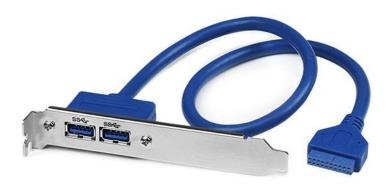
The USB3SPLATE 2-Port USB 3.0 A Slot Plate converts the USB pins on the USB 3.0 motherboard header to 2 standard USB 3.0 A-type ports. The plate can be mounted on the rear panel of a computer case, adding two USB 3.0 A female ports for simple connection to USB peripheral devices.
